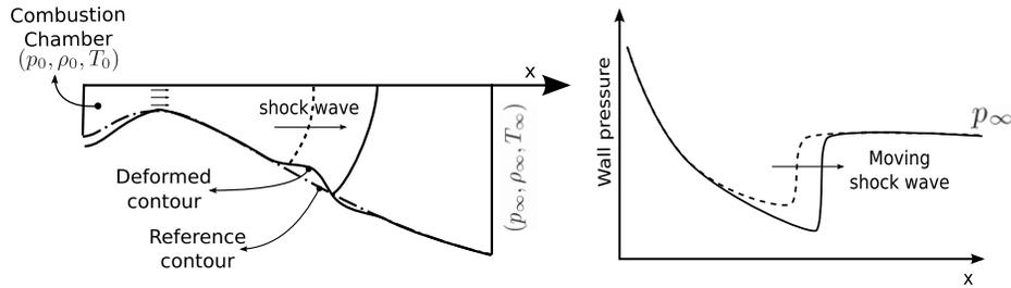
Figure 9: Schematic deformation of the structure.
