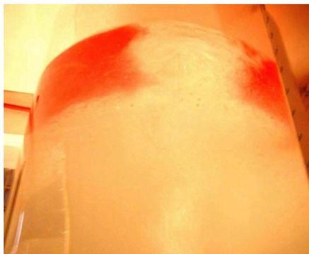
Figure 7: Lateral view of the ladle when two plugs are used, where one of the open eyes in contact with the wall can be seen.
