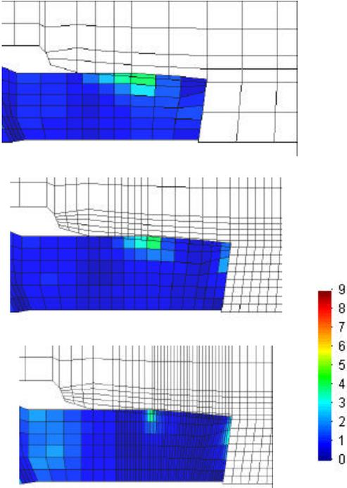
Figure 5: Refinement indicator for the region of the sealing.
