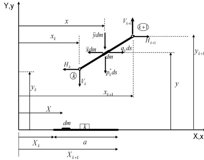
Figure 2: Free forces diagram of a generic link
