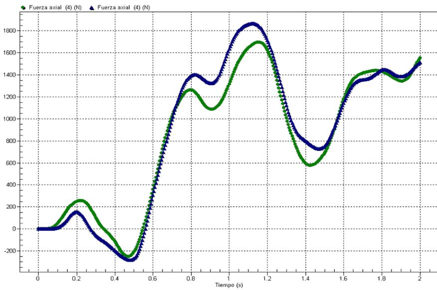
Figure 11: Illustration example 2. Axial forces at the fourth node.(FEM solution).
