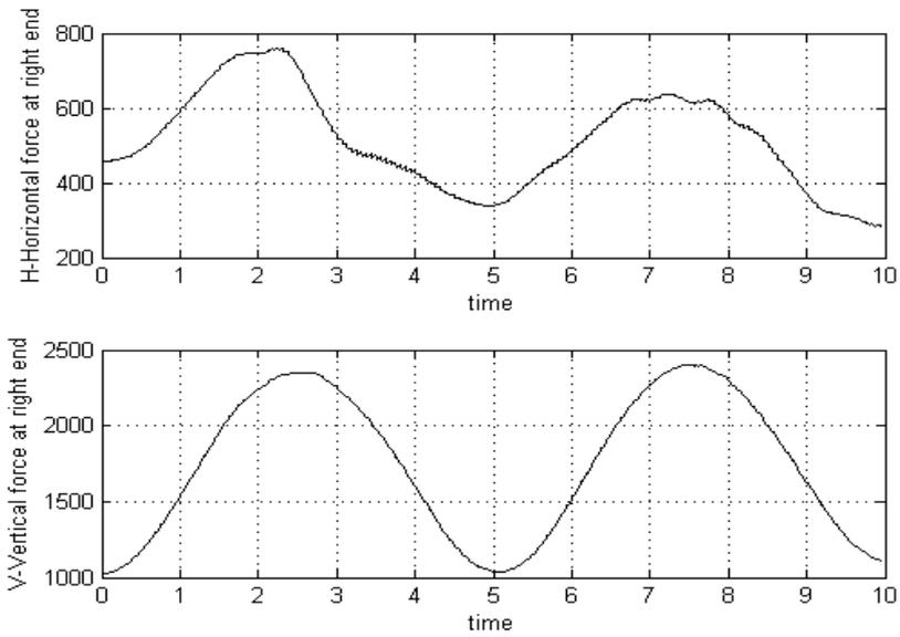
Figure 6: Illustration example 1. Horizontal and vertical forces at right-end of chain.
