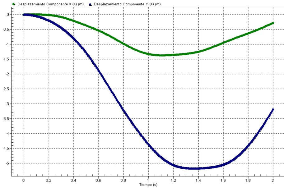
Figure 10: Illustration example 2. Horizontal and vertical displacement at the fourth node.(FEM solution).
