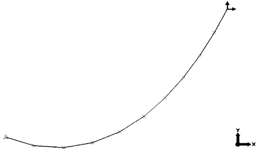
Figure 3: Illustration examples 1 and 2. Initial configuration for the chain (Nodes coordinates depicted in Table 1)
