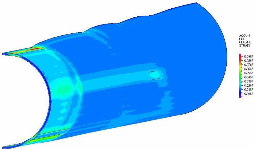
Figure 7: Accumulated effective plastic strain, external view.
