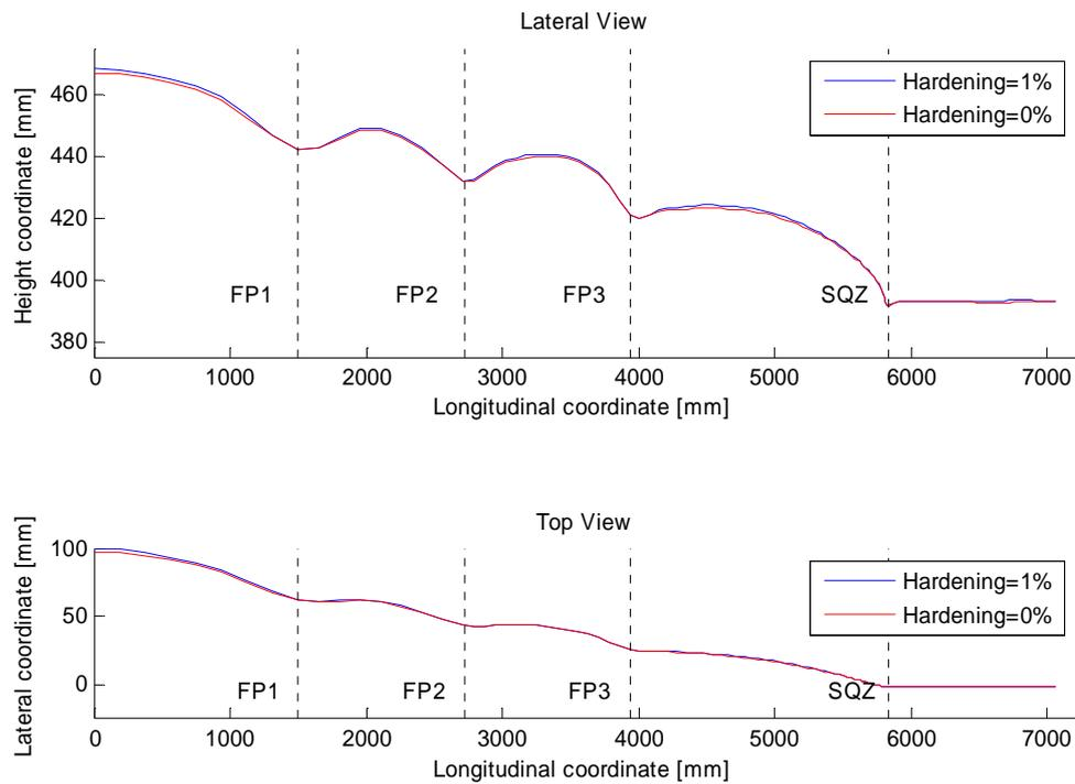
Figure 11: Skelp edge position. Lateral and top view.
