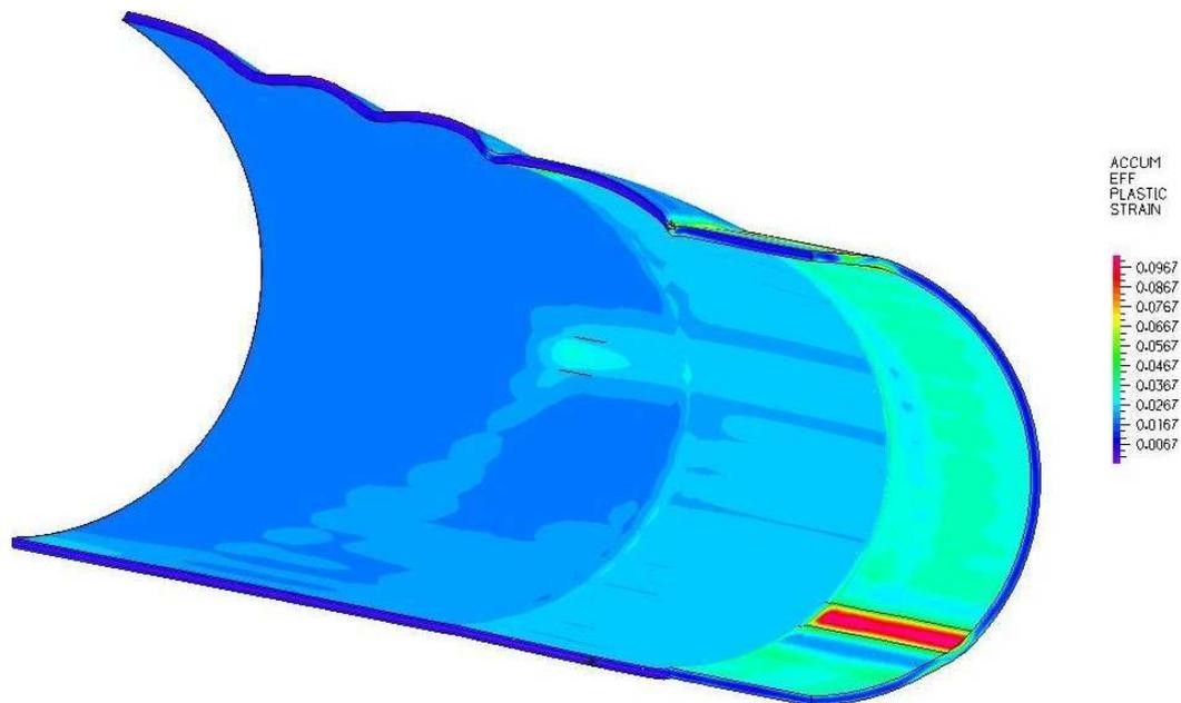
Figure 8: Accumulated effective plastic strain, internal view.
