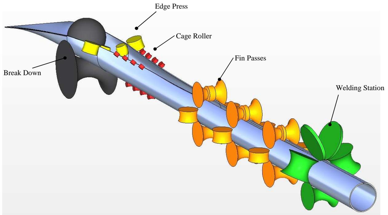
Figure 1: Schematic diagram of an ERW line.
