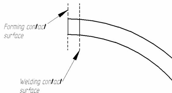
Figure 4: Forming and welding contact surfaces.
