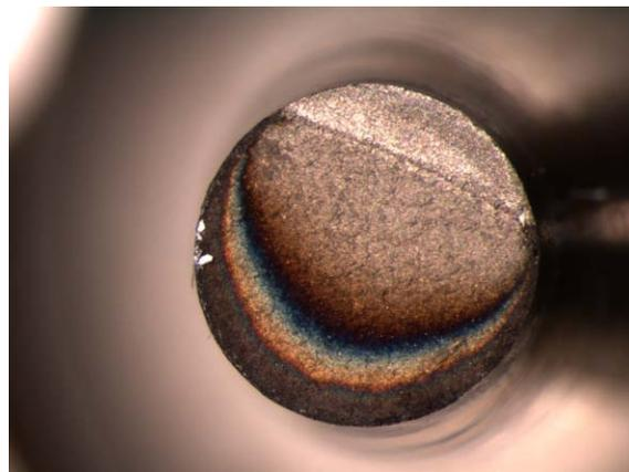
(b) Fracture surface of the specimen failed at 337MPa in  $1.85 \times 10^5$  cycles at 20°C.
