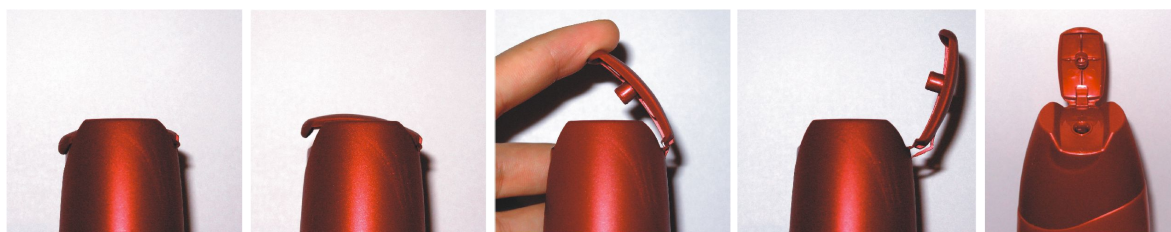
Figure 1: Bistable mechanism of a shampoo bottle lid: human intervention is needed to unlock and guide the lid until surpassing the angular unstable position, in the middle photograph; then, the internal strain energy stored in the flexible members drives the lid to the final stable position.
