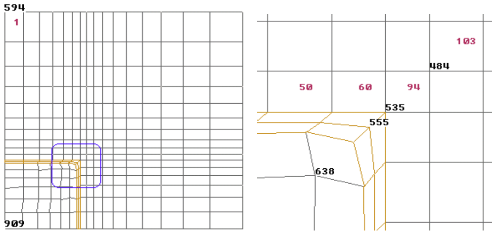
Figure 6: Mesh used for the numerical analysis (1/4 of the whole problem) and detail of the internal corner. Nodes and elements numbered are those for which plots are presented
