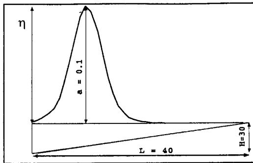
Figure 2: Coordinate system for shallow water equations.
