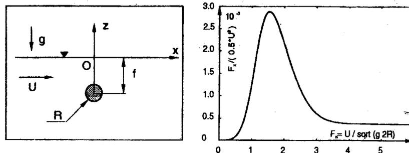
Figure 7: wave drag as a function of the Froude number for a horizontal circular cylinder obtained by the extended panel method.
