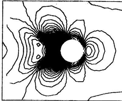
Figure 8: isolines of elevation for a semi submerged sphere at Froude number  $F = 4.5$ .
