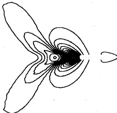
Figure 9: isolines of elevation for a scale ship model at Froude number  $F = 0.5$ .
