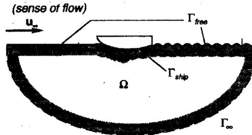
Figure 1: ship-like body with constant forward velocity in a infinitely deep and calm uniform sea.
