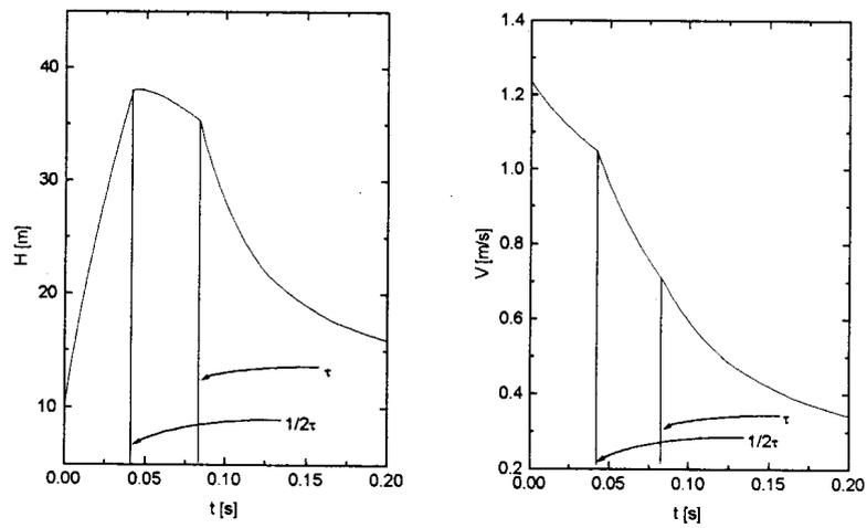
Figure 5. Evolution of  $H$  and  $V$  at the valve inlet (node 11)
