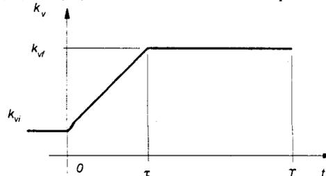
Figure 2. Time variation of the valve friction coefficient.
