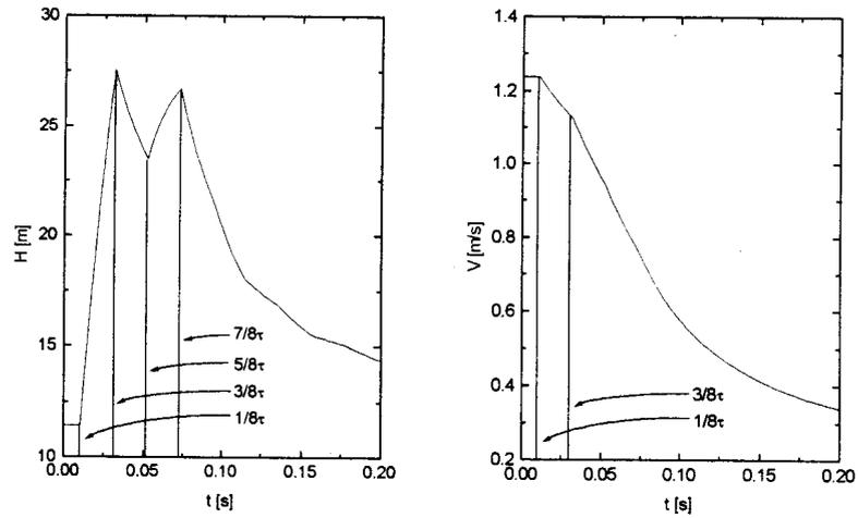
Figure 4. Evolution of  $H$  and  $V$  at the middle of the pipe (node 6)
