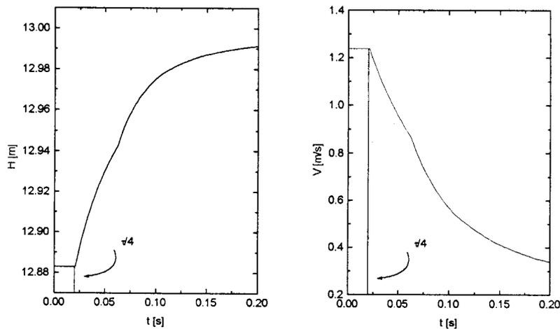
Figure 3. Evolution of  $H$  and  $V$  at the tank outlet (node 1)
