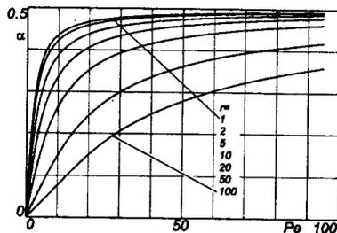
Figure 3: Proportionality constant for the standard SUPG perturbation term  $\alpha$  as function of  $Pe$  for constant  $r$ .
