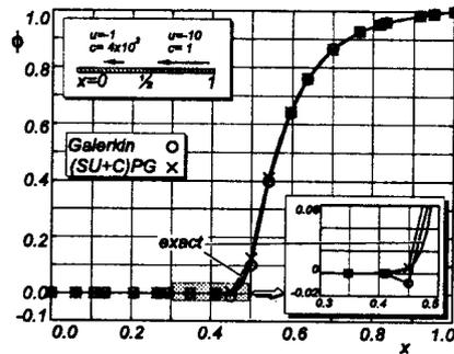
12: Example with non-constant physical properties. Comparison between the different methods.
