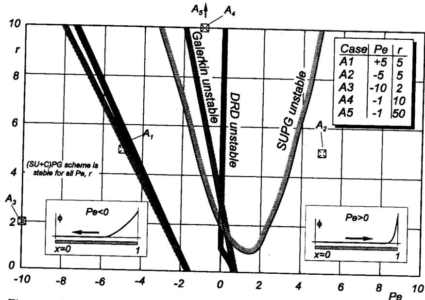
Figure 6: Experimentally determined stability map for Galerkin, DRD and SUPG.
