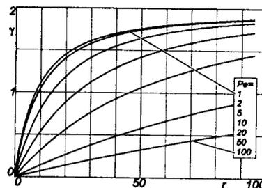
Figure 4: Proportionality constant for the second perturbation function  $\gamma$  as function of  $r$  for constant  $Pe$ .
