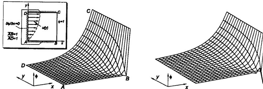
14: Two-dimensional example with advection (parabolic profile). Problem description and numerical results with the (SU+C)PG scheme.
