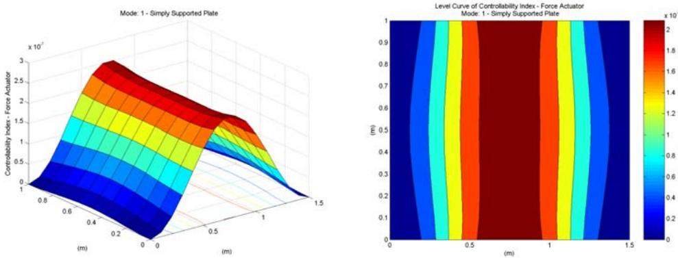
Figure 5 – Force actuator placement index for 1<sup>o</sup> mode (a) Surface (b) Level contour.
