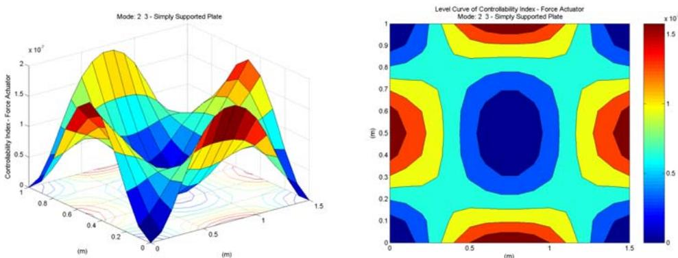
Figure 9 – Force actuator placement index for 2 and 3 modes (a) Surface (b) Contour level.
