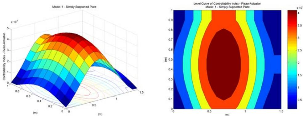
Figure 6 – Piezoactuator placement index for 1<sup>o</sup> mode (a) Surface (b) Level contour
