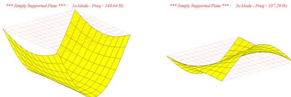
Figure 3 – Vibration shapes (a) 1<sup>o</sup> Mode (b) 2<sup>o</sup> Mode.
