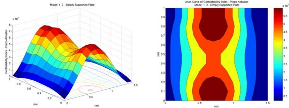
Figure 8 – Piezoactuator placement index for 1 and 2 modes (a) Surface (b) Contour level.
