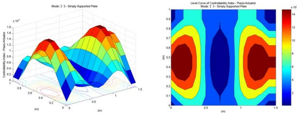
Figure 10 – Piezoactuator placement index for 2 and 3 modes (a) Surface (b) Contour level.
