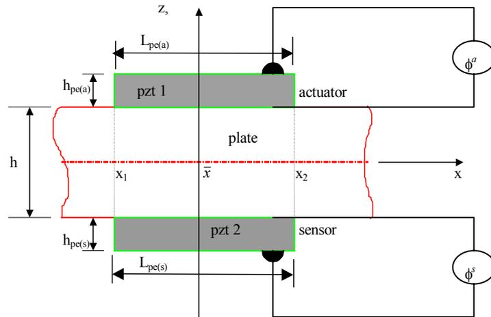
Figure 2 – Plate with piezoelectric elements attached (Lima Jr & Arruda, 1999).
