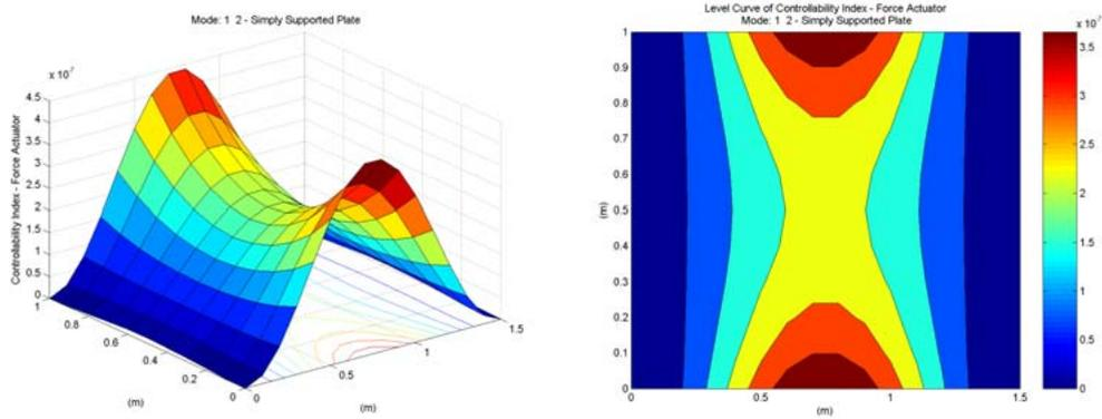
Figure 7 – Force actuator placement index for 1 and 2 modes (a) surface (b) Contour level.
