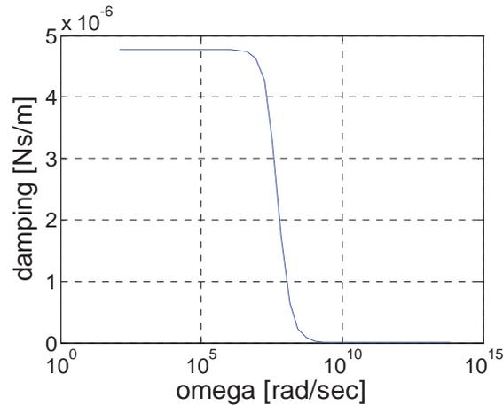
Figure 3: Damping component of the damping coefficient for the rigid plate problem
