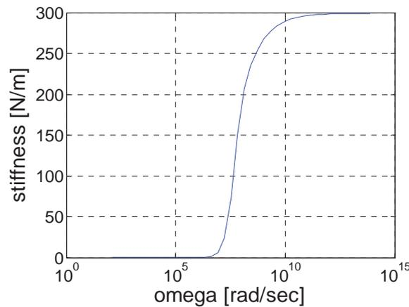
Figure 4: Stiffness component of the damping coefficient for the rigid plate problem
