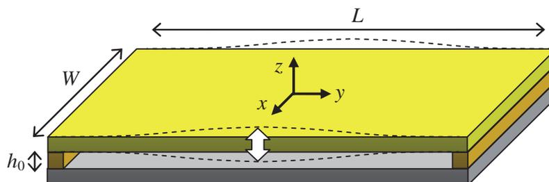
Figure 1: Schematic representation of a vibrating microplate over a substrate.
