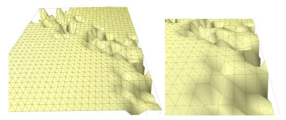
Figure 2: Regular grid data discretization (river section and detail)
