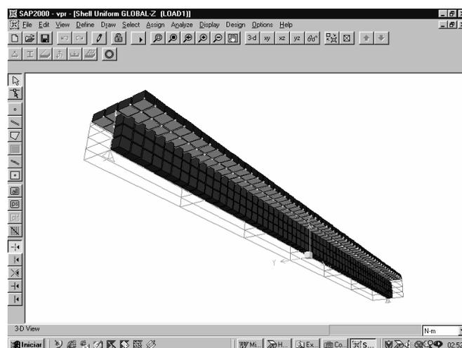
Figure 5- Mesh used to characterize the mixed beam in SAP 2000
