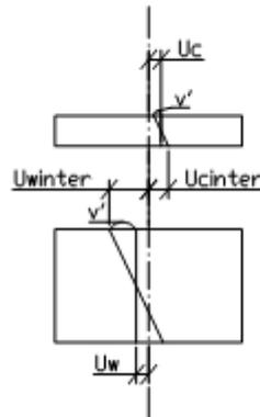
Figure 6 - Kinematics of a composite beam
