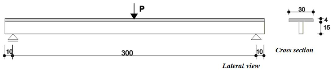
Figure 3 – Dimensions of Composite Beam (cm)
