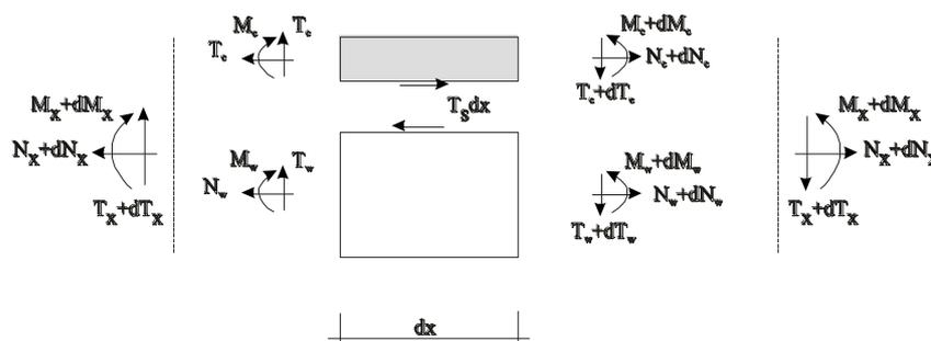
Figure 2 - Representation of the internal efforts in concrete and wood
