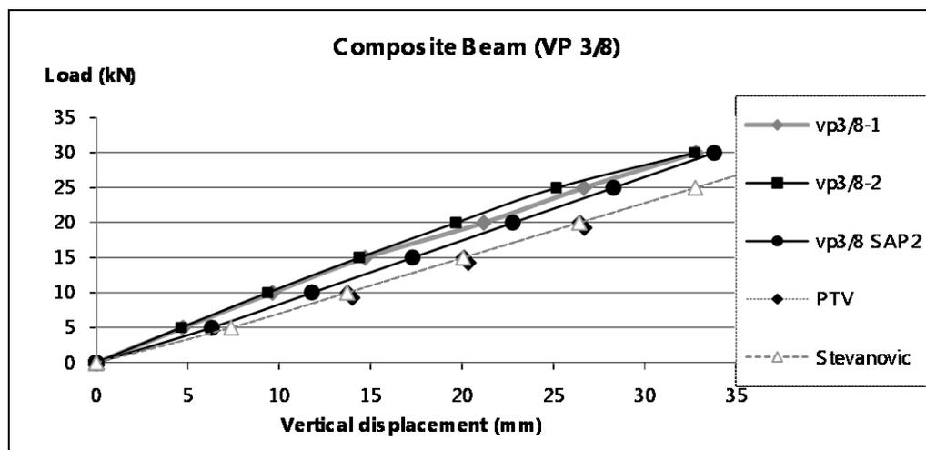
Figure 7 - Results of the vertical displacement 1/3 of the beam span
