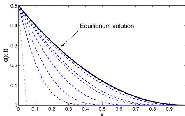
Figure 3: The plot represents the simulation of the first phase of the oxygen diffusion problem. Oxygen concentration at different times: the initial concentration (dotted), some iterations (dashed) and the equilibrium solution given by (11) (solid).
