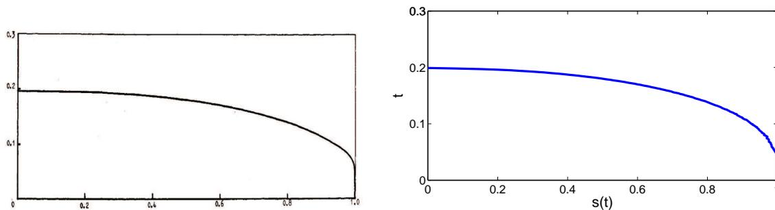
Figure 5: Both plots represent the moving boundary position  $s(t)$  on the horizontal coordinate and time  $t$  on the vertical one. The left Figure corresponds to the results obtained in (Crank and Gupta, 1972) and the right Figure corresponds to our simulations.
