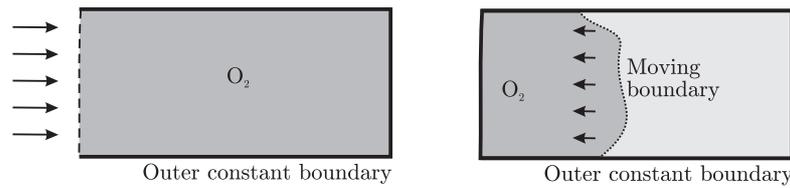
Figure 1: Schematic representation of the oxygen diffusion into the media sample. The first stage is represented on the left. Here the oxygen enters the sample until equilibrium is reached. During the second phase, on the right, the sample is sealed and the oxygen inside diffuses and is absorbed by the medium generating the moving boundary.
