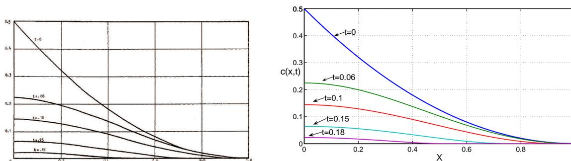
Figure 4: Both plots represent the simulation of the second phase of the oxygen diffusion problem. The oxygen concentration is represented for different times (from upper to lower)  $t = 0$ ,  $t = 0.06$ ,  $t = 0.1$ ,  $t = 0.15$  and  $t = 0.18$ . The left Figure corresponds to the results obtained in (Crank and Gupta, 1972); the right Figure corresponds to our simulations.
