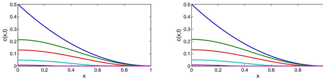
Figure 6: Both plots represent the simulation of the second phase of the non-linear oxygen diffusion problem. The oxygen concentration is represented for different times (from upper to lower)  $t = 0$ ,  $t = 0.06$ ,  $t = 0.1$ ,  $t = 0.15$  and  $t = 0.18$ . Left Figure corresponds to the results obtained using the (FDA-NCP); the right Figure corresponds to the classical Crank-Nicolson scheme.
