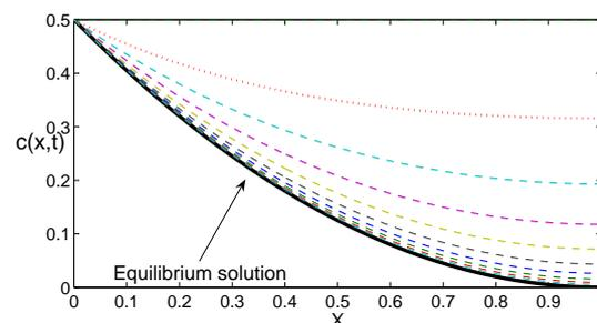
Figure 2: The plot represents the simulation of the first phase of the oxygen diffusion problem. Oxygen concentration at different times: the initial concentration (dotted), some iterations (dashed) and the equilibrium solution given by (11) (solid).
