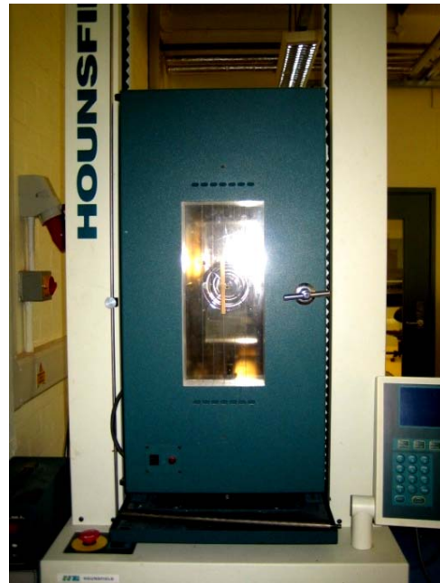
Figure 10: Tension test at elevated temperature: Chamber where specimen is placed in.
