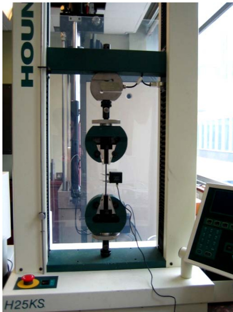
Figure 9: Tension test at room temperature: Clamped specimen with attached extensometer.
