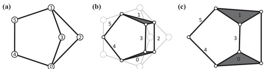
Figure 7: Direct sketching of the kinematic chain and refinement using a force-based algorithm.
