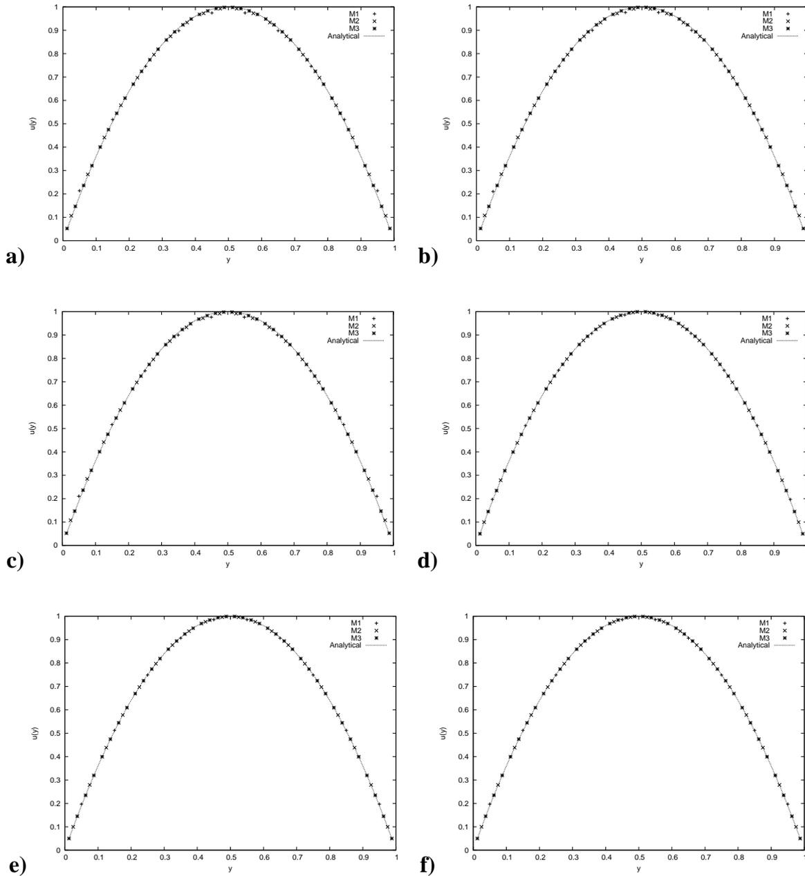
Figure 2: Comparison between numerical solutions obtained by  $P1$  and  $P2$  methods using  $IF$  and analytical solution, over three grids and  $Re = 0.1$ . **a)-c)**  $P1$  method using the formulations  $BI$ ,  $CN$  and  $AB/CN$ , and **d)-f)**  $P2$  method using the formulations  $BI$ ,  $CN$  and  $AB/CN$ , respectively.
