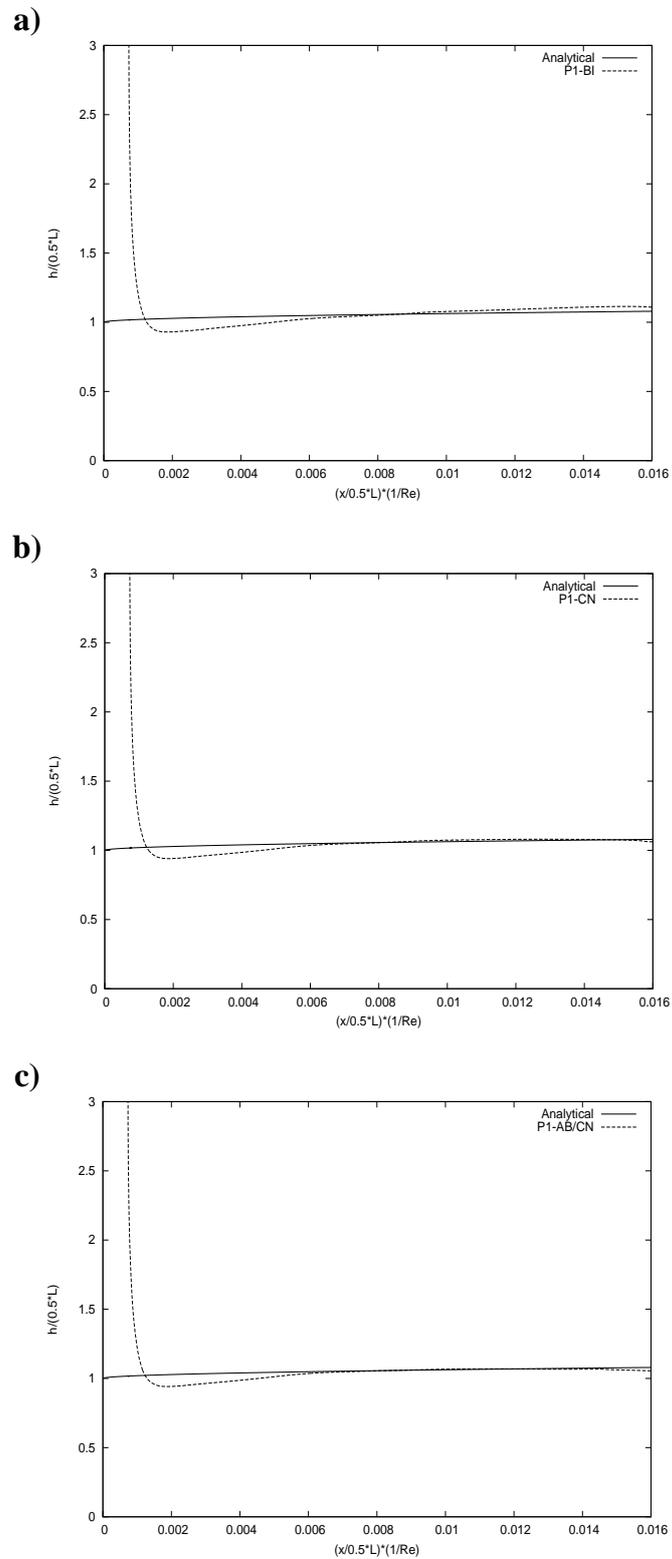
Figure 3: Comparison between Watson’s exact solution and the numerical solution for the impinging jet, with  $Re = 5 \times 10^3$  : a)-c)  $P1$  method using the formulations  $BI$ ,  $CN$  and  $AB/CN$ , respectively.
