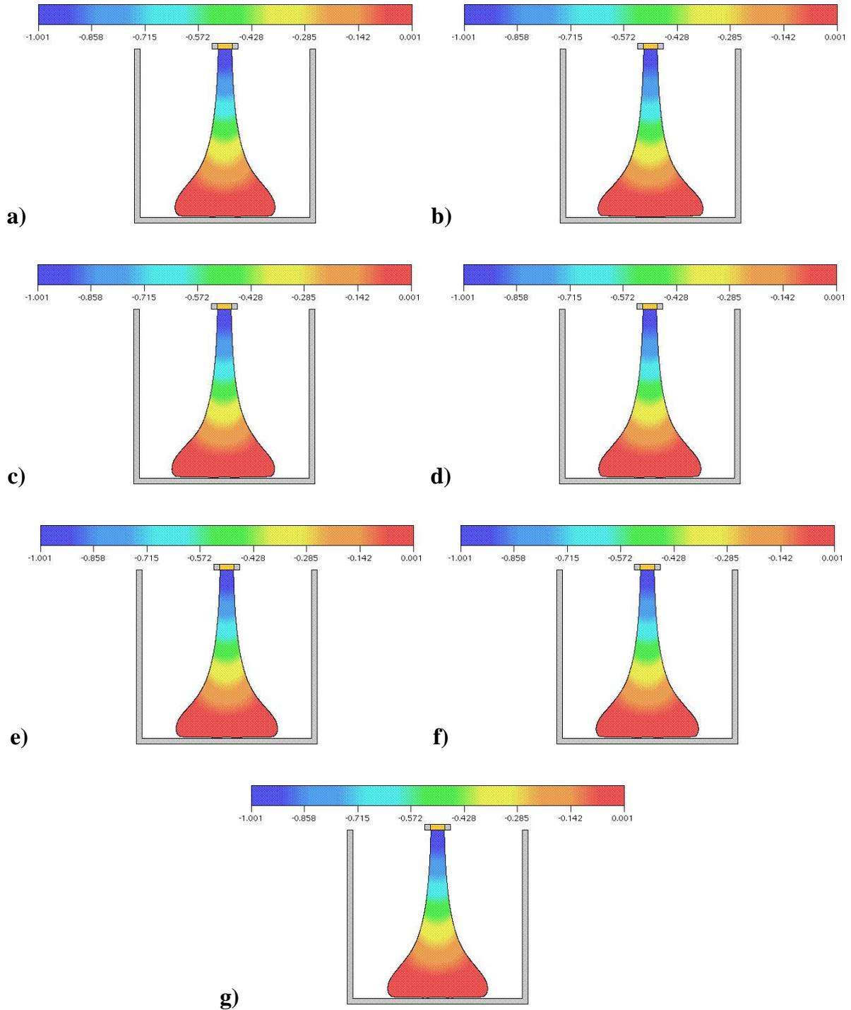
Figure 8: Comparison of velocity field  $v$  for  $t = 0.14s$ . Methods: **a)** Explicit, **b)-d)**  $P1$  using the  $BI$ ,  $CN$  and  $AB/CN$  formulations, respectively, and **e)-g)**  $P2$  using the  $BI$ ,  $CN$  e  $AB/CN$  formulations.
