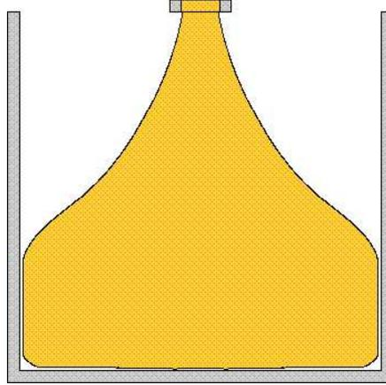
Figure 5: Numerical simulation of container filling, with  $Re = 0.1$  and simulation time  $t = 0.28s$ , for the  $P2$  method using the  $CN$  formulation.
