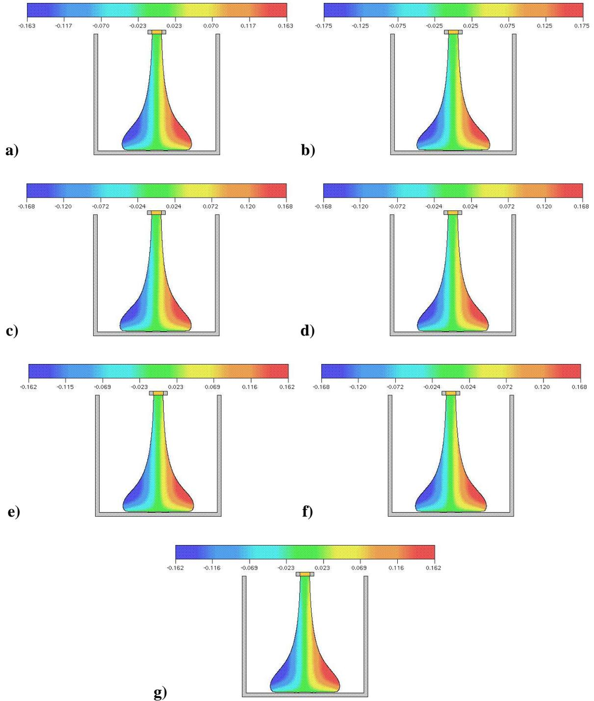
Figure 7: Comparison of velocity field  $u$  for  $t = 0.14s$ . Methods: **a)** Explicit, **b)-d)**  $P1$  using the  $BI$ ,  $CN$  and  $AB/CN$  formulations, respectively, and **e)-g)**  $P2$  using the  $BI$ ,  $CN$  e  $AB/CN$  formulations.
