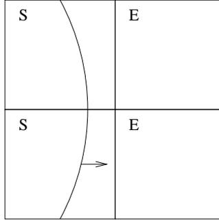
Figure 1: Configuration of a computational cell showing a free surface cells in contact, on its right hand face, with an empty cell.
