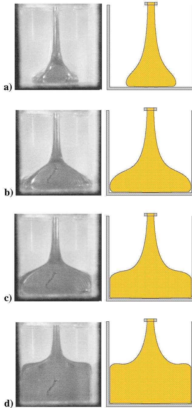
Figure 6: Experimental solution (left) and numerical (right) solution by using  $P2$  method with the  $BI$  formulation. **a)**  $t = 0.14$ s, **b)**  $t = 0.22$ s, **c)**  $t = 0.26$ s and **d)**  $t = 0.34$ s.
