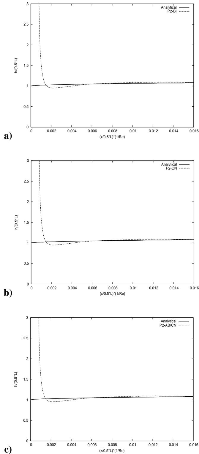
Figure 4: Comparison between Watson's exact solution and the numerical solution for the impinging jet, with  $Re = 5 \times 10^3$  : a)-c) P2 method using the formulations *BI*, *CN* and *AB/CN*, respectively.
