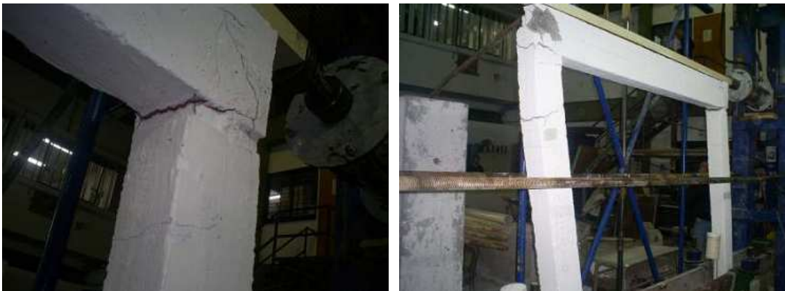
Figure 3: Frame1 after the test
