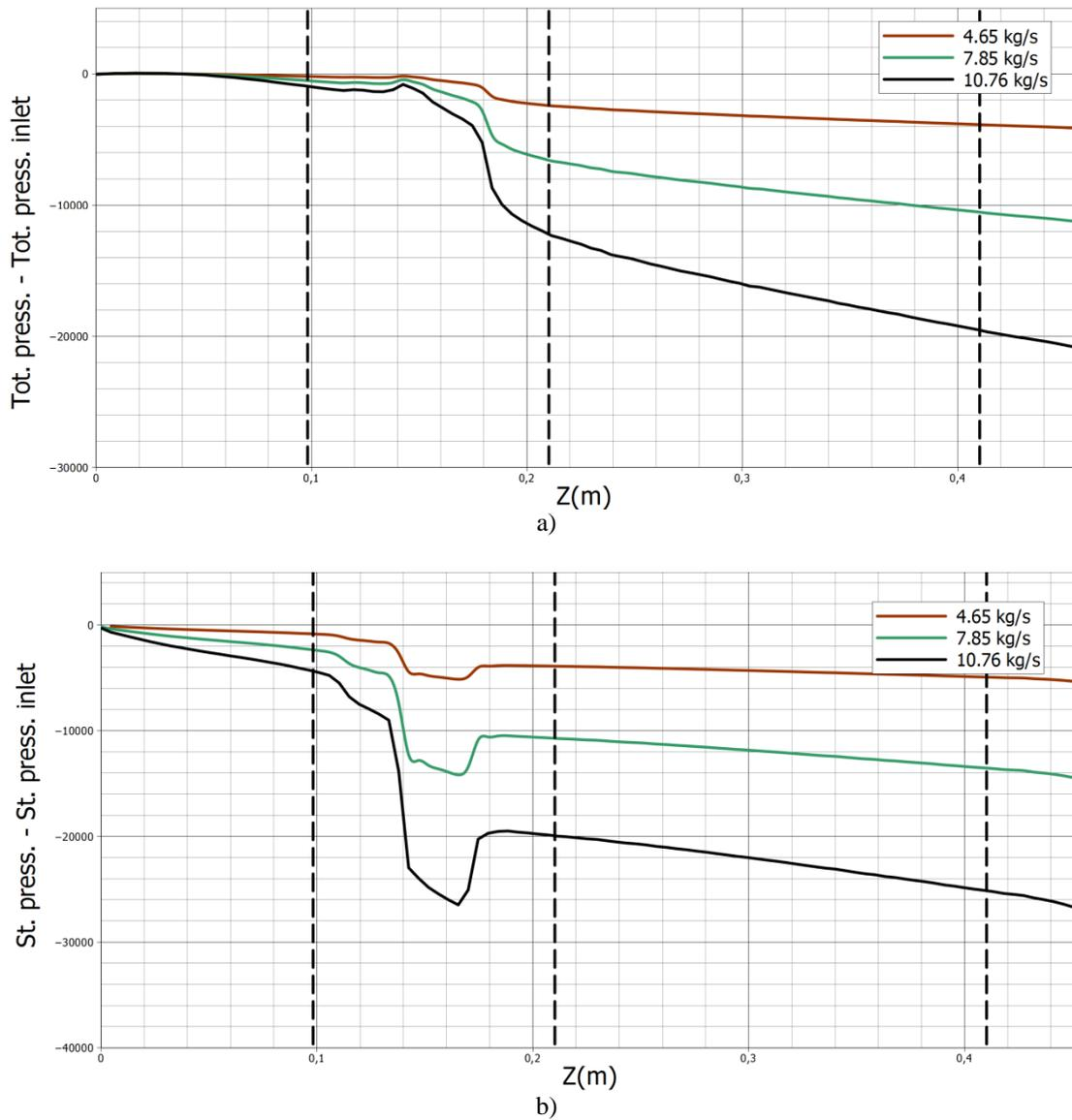
Figure 2: Pressure distribution along fuel assembly for different mass flow rates. a) Total pressure; b) static pressure.
