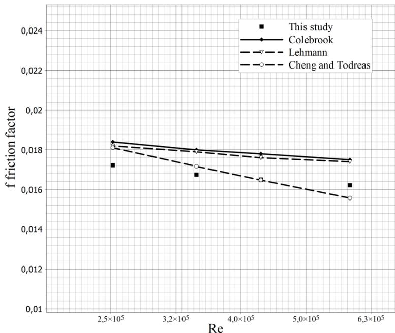
Figure 3: Friction factor
