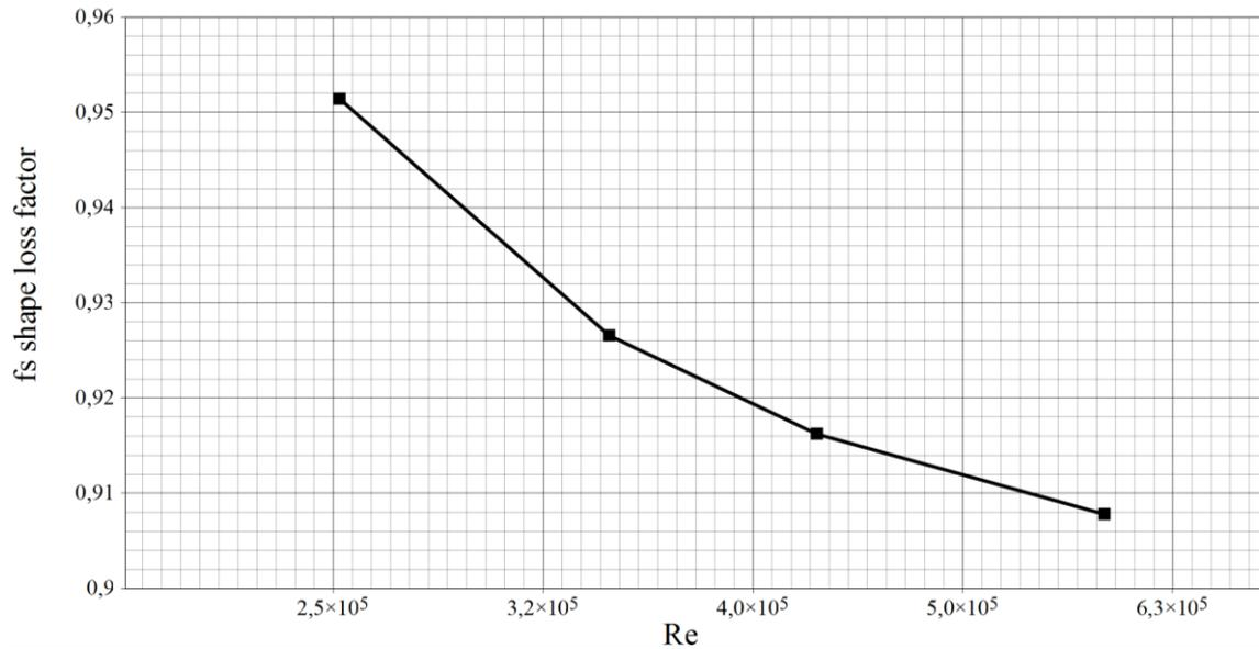
Figure 5: Spacer form factor vs. Re numbers
