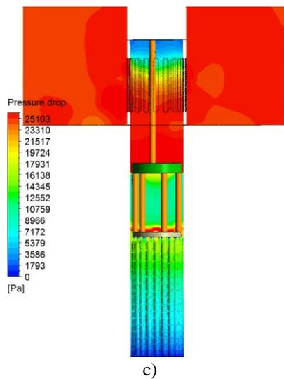
Figure 8: Pressure distribution in fuel channel throttles a) Total pressure; b) Static pressure; c) Contour of static pressure shown over fuel channel throttles geometry.
