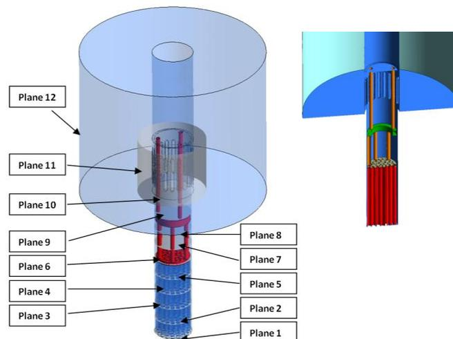
Figure 7: Geometry details for fuel channel throttles
