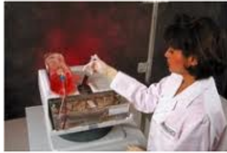
Figure 4. Bioreactor for stem cells propagation (Aastrom Inc, Ann Arbor, MI, USA).
