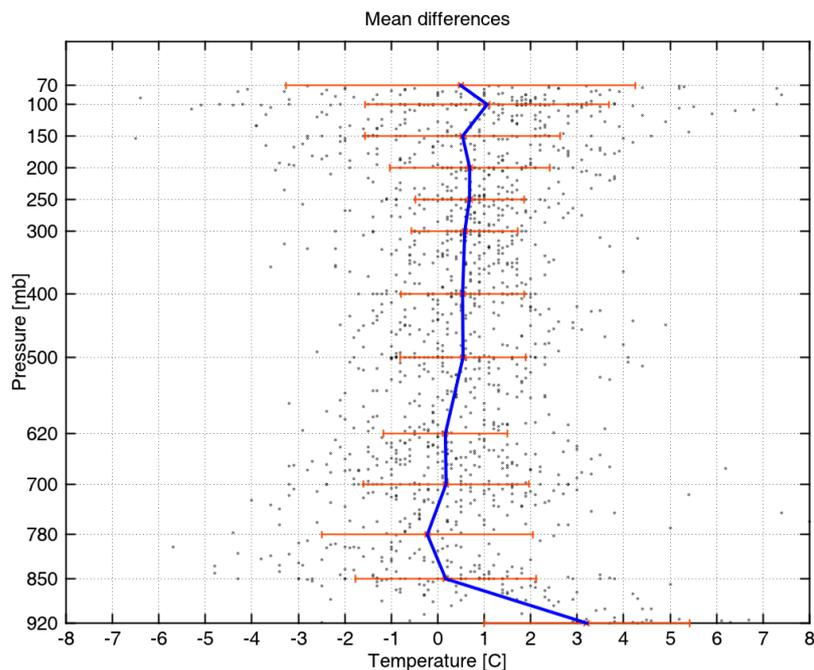
Figure 8: Mean differences and standard deviation between WRF and radiosonde temperature profiles, for 2007 summer days.
