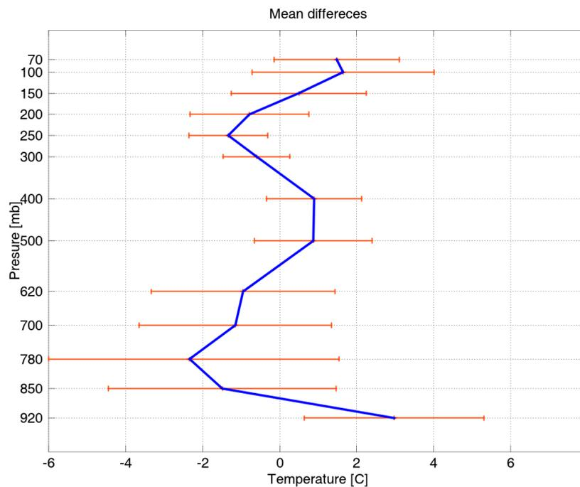
Figure 9: Mean differences between WRF and MODIS temperature profiles over the whole domain for February 20, 2007. Orange bars represent the standard deviation.
