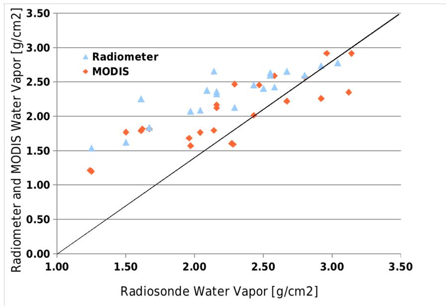
Figure 5: Correlation between Radiometer, MODIS and radiosondes, for 2007 radiometer measurement campaign in Mendoza.
