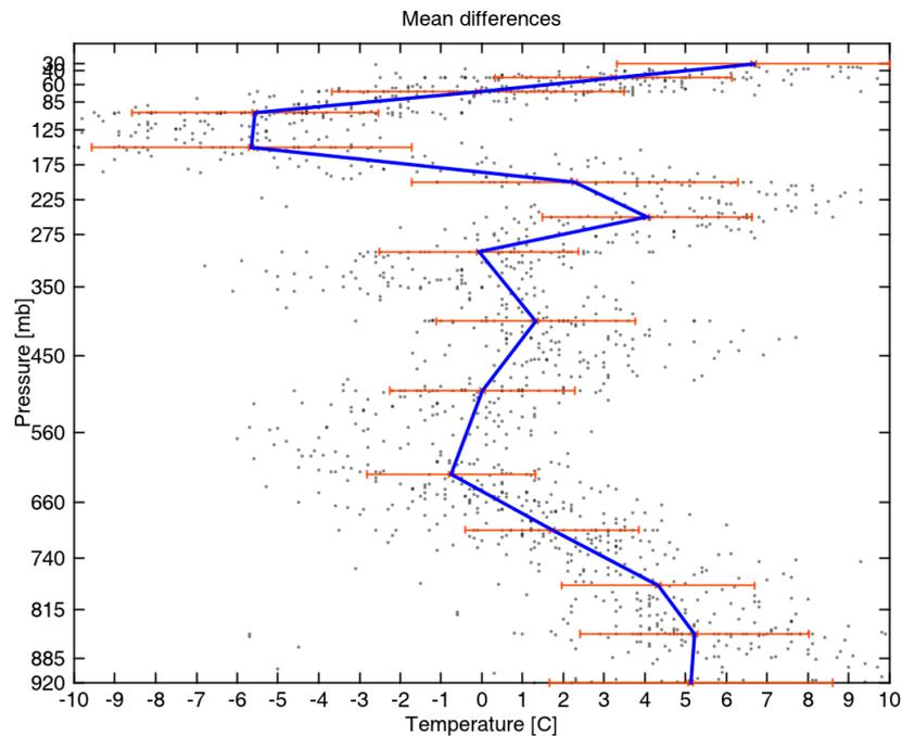
Figure 2: Mean differences (blue line) between MODIS and radiosonde 2007 profiles, and standard deviation (orange bars). Black dots represent absolute differences. Averaging kernel radius  $r=0$ .
