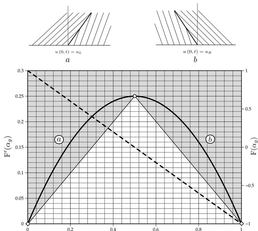
Figure 3: Riemann problem solutions for a convex flux. a. Right going shock, b. left going shock. — flux, - - - flux derivative
