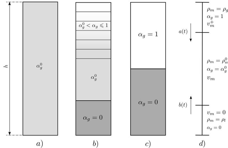
Figure 2: Simple sedimentation experiment. a) Initial conditions; b) settling transitory; c) steady state and d) simple scheme of problem variables
