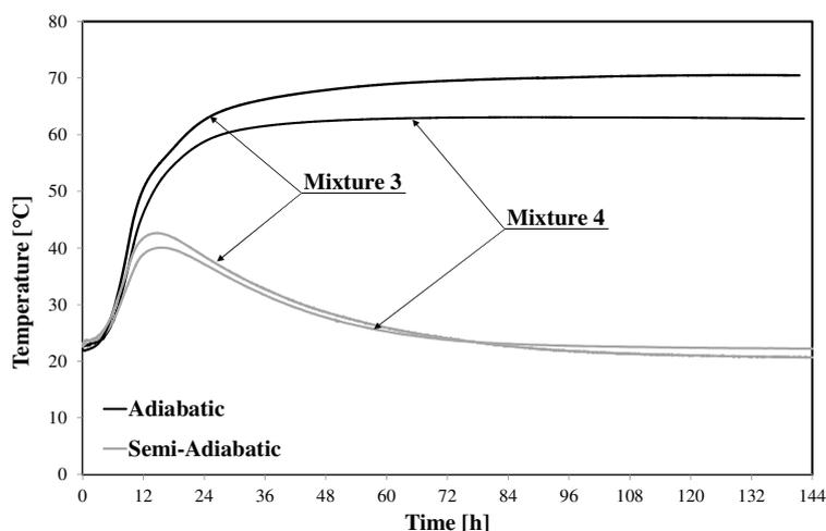
Figure 4: Experimental results: time evolution of temperature by Koenders (2005).
