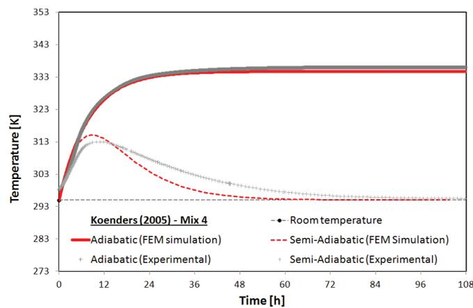
Figure 9: Comparison between the experimental data by Koenders (2005) and the FEM based results (adiabatic heat production according to Eq. (5)): Mixture 4.
