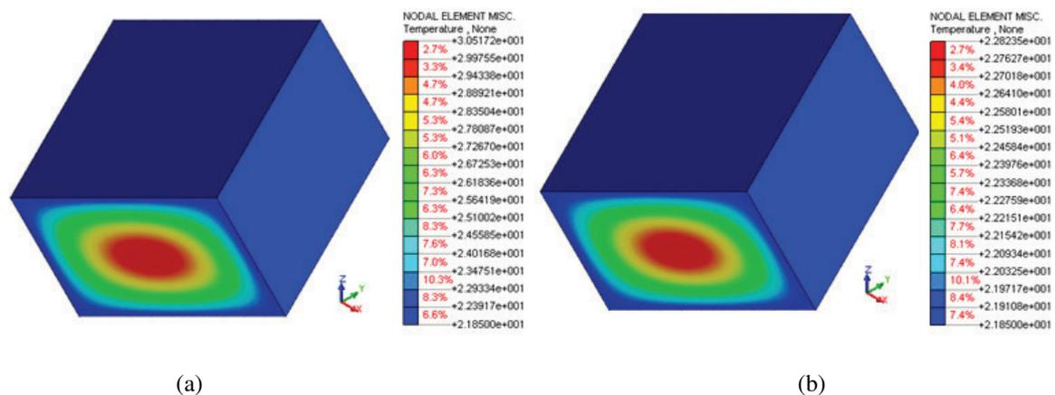
Figure 11: Temperature evolutions [ $^{\circ}\text{C}$ ] of the Mixture 4 in non-adiabatic condition: (a) after 24 h and (b) after 48 h.
