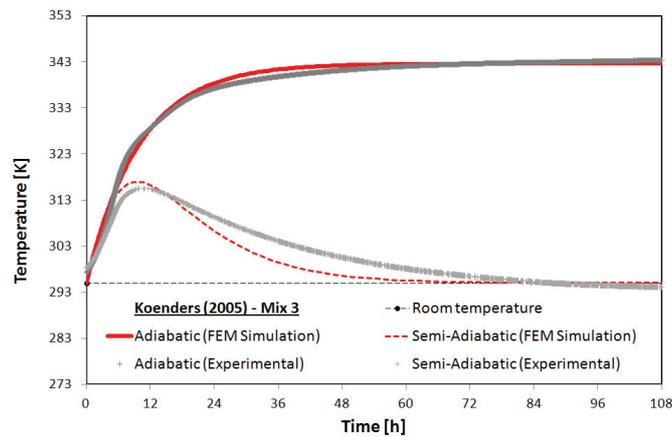
Figure 8: Comparison between the experimental data by Koenders (2005) and the FEM based results (adiabatic heat production according to Eq. (5)): Mixture 3.
