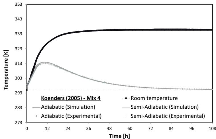
Figure 6: Comparison between the experimental data by Koenders (2005) and the theoretical results of the time evolution of Temperature (adiabatic heat production according to Eq. (5)): Mixture 4.
