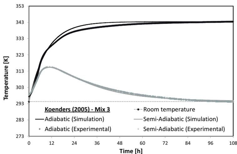
Figure 5: Comparison between the experimental data by Koenders (2005) and the theoretical results of the time evolution of Temperature (adiabatic heat production according to Eq. (5)): Mixture 3.
