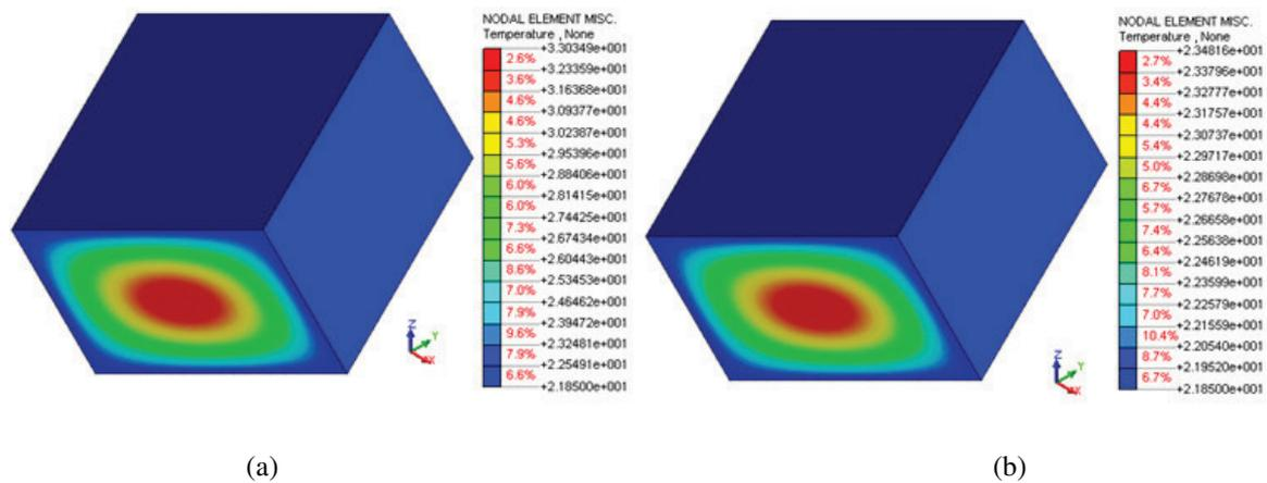
Figure 10: Temperature evolutions [ $^{\circ}\text{C}$ ] of the Mixture 3 in non-adiabatic condition: (a) after 24 h and (b) after 48 h.
