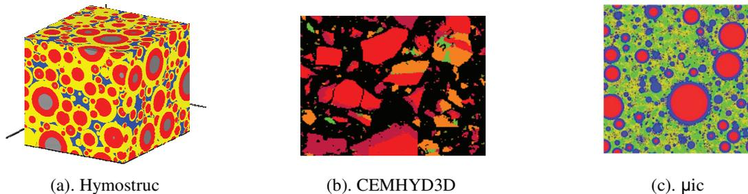
Figure 1: Impression of three advanced hydration models that operate at the micro-scale level: (a) Hymostruc (van Breugel, 1991), (b) CEMHYD3D by Bentz et al. (1993) and (c)  $\mu$ ic by Bischnoi (2008).
