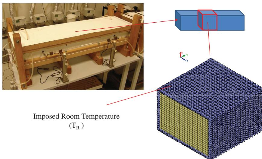
Figure 7: Geometry and boundary conditions of the FEM problem according to Koenders (2005) tests.
