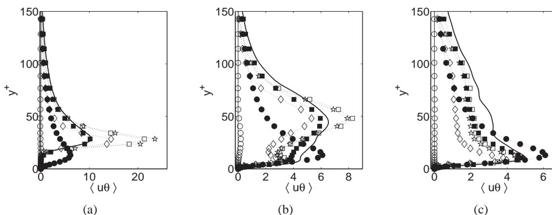
Figure 4: A priori comparison of modeled  $\langle u\theta \rangle$  with DNS data, for channel flow perturbed with blowing for  $Pr = 1$ . Filled circles, non-perturbed flow; filled squares, DNS data; solid line, present model;  $\circ \cdot \circ \cdot \circ$ , SGDF;  $\square \cdot \square \cdot \square$ , GGDH;  $\star \cdot \star \cdot \star$ , HoGGDH;  $\diamond \cdot \diamond \cdot \diamond$ , YSC. (a) on the slot; (b)  $1.5W^+$  and (c)  $5W^+$  from the slot. Note the different scales.
