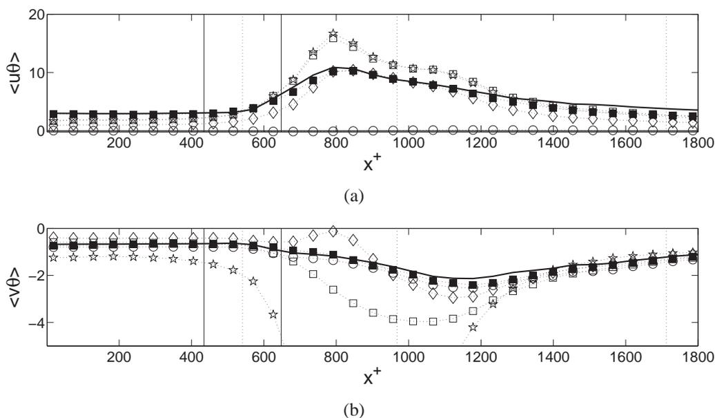
Figure 8: Idem Fig. 4(a)-4(c), but along  $x^+$  at  $y^+ = 38$ . (a)  $\langle u\theta \rangle$ ; (b)  $\langle v\theta \rangle$ . Note the different scales. Solid vertical lines denote the slot location, vertical dotted lines denote sections on the middle of the slot, and at  $1.5W^+$  and  $5W^+$  from the slot. Note also that the scale does not include extreme over predictions.
