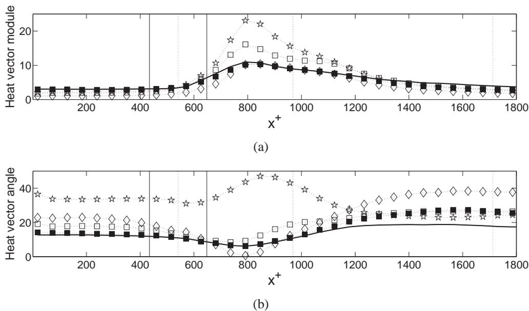
Figure 10: *A priori* comparison of the (a) module and (b) angle (degree) regarding to the horizontal, of the heat flux vector with DNS data, for channel flow perturbed with blowing. Filled squares, DNS data; solid line, present model;  $\square \cdot \square \cdot \square$ , GGDH;  $\star \cdot \star \cdot \star$ , HoGGDH;  $\diamond \cdot \diamond \cdot \diamond$ , YSC.
