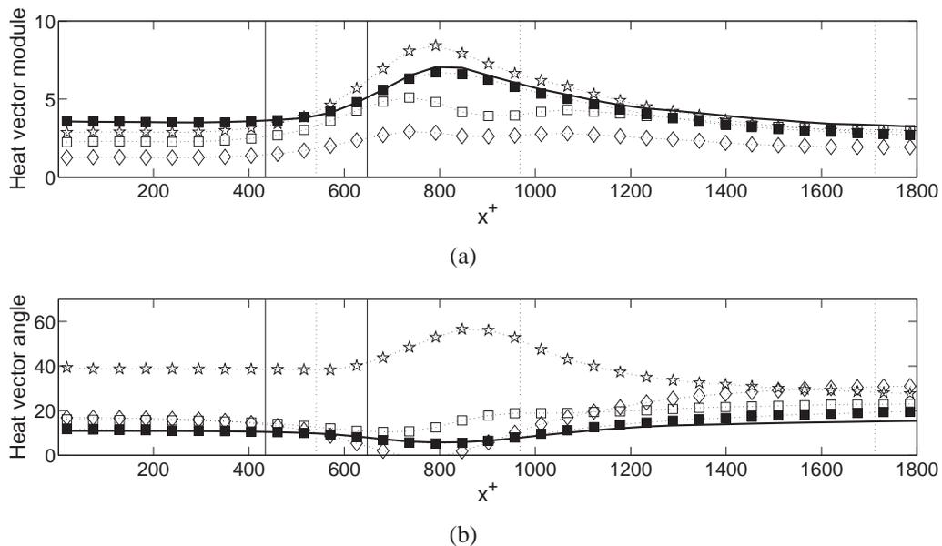
Figure 11: Idem Figs. 10(a) and 10(b) for channel flow perturbed with an APGS. (a) module; (b) angle (degree).
