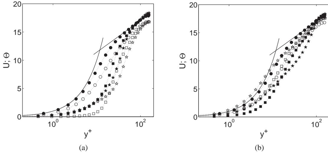
Figure 1:  $U$  (filled symbols) and  $\Theta$  (open symbols) for channel flow perturbed with (a)blowing and an (b)APGS, on the slot (squares) and  $W^+$  downstream from the slot (stars). Open and filled circles  $U$  and  $\Theta$  for non-perturbed flow, respectively. Solid line, law of the wall,  $(1/0.41)\ln(y^+) + 5.0$ .
