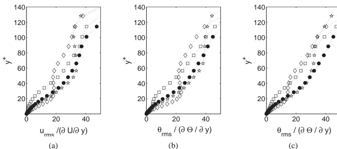
Figure 3: (a)  $u_{rms}/(\partial U/\partial y)$ ; (b)  $\theta_{rms}/(\partial \Theta/\partial y)$  for  $Pr = 1$ ; (c)  $\theta_{rms}/(\partial \Theta/\partial y)$  for  $Pr = 0.5$  for channel flow perturbed with blowing. Filled circles non-perturbed flow;  $\square \cdot \square \cdot \square$  on the slot;  $\diamond \cdot \diamond \cdot \diamond$   $1.5W^+$ ;  $\star \cdot \star \cdot \star$   $5W^+$  downstream of slot.
