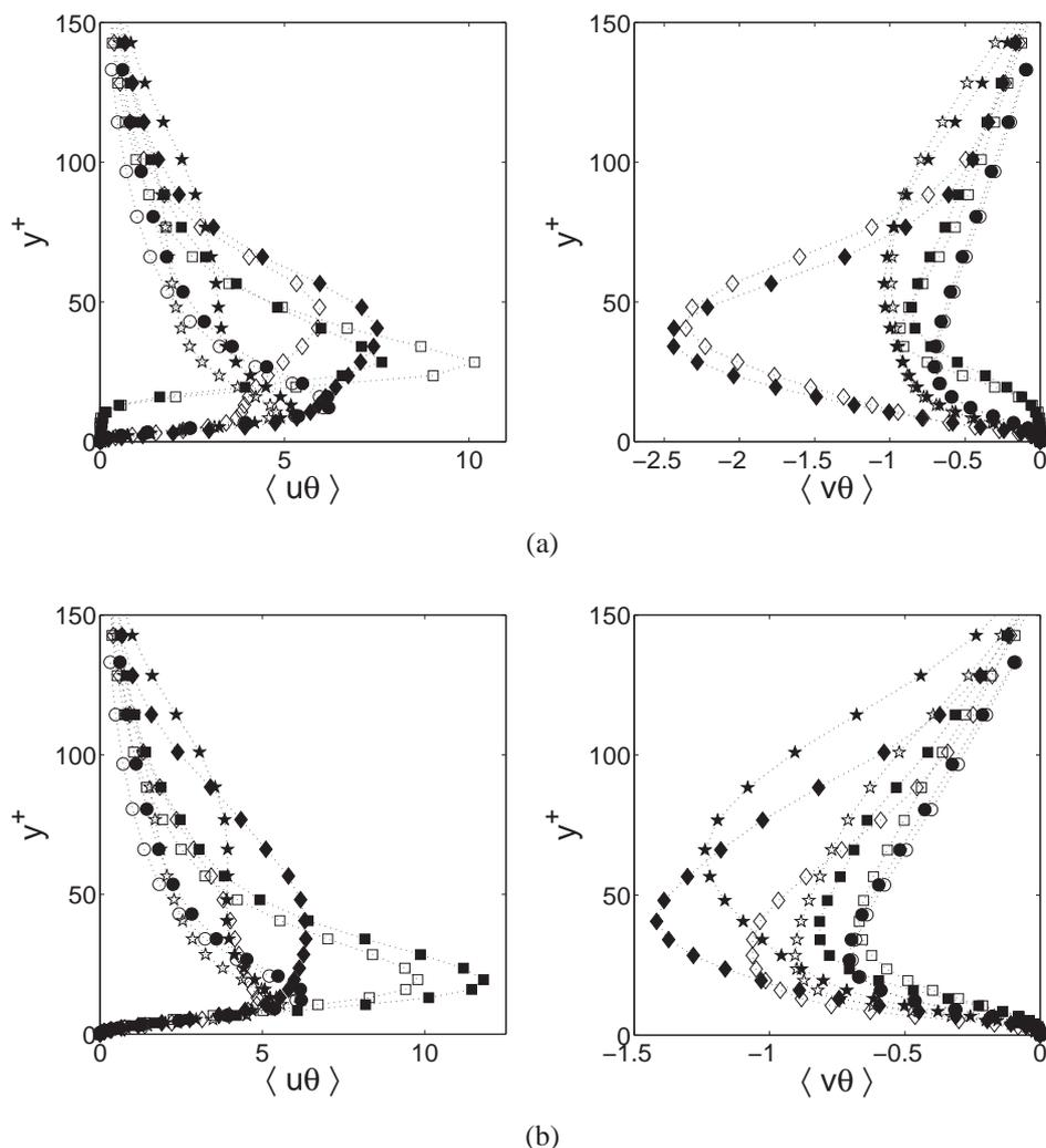
Figure 2: DNS values of  $\langle uv \rangle$  and  $\langle u\theta \rangle$  (filled symbols); and  $\langle v\theta \rangle$  (open symbols), for channel flow perturbed with (a) blowing and (b) APGS for  $Pr = 1$ . Circles, non-perturbed flow; squares, on the slot; diamonds, at  $1.5W^+$  and stars  $5W^+$  downstream from the slot. Note the different scales.
