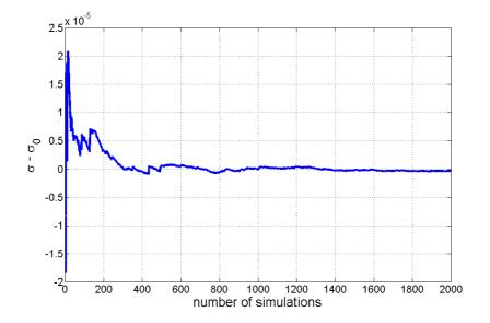
Figure 9: Collision between two spheres. Convergence study of the time of contact using the Monte Carlo method.  $\sigma$  and  $\sigma_0$  correspond to the standard deviation found with the numerical simulation and the analytical approach, resp.
