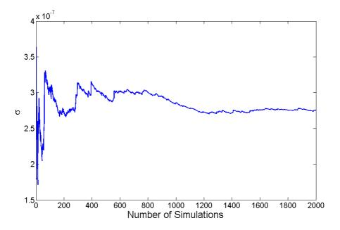
Figure 14: Collision between two discs. Convergence study of the standard deviation of the time of contact with Monte Carlo simulations.
