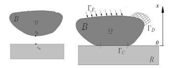
Figure 12: Scheme of the contact of a deformable body against a rigid contact.
