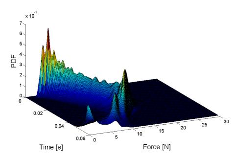
Figure 19: Idem Fig.17. Evolution of the probability density function of the interaction force.
