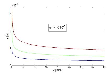
Figure 6: Curves  $\tau$  vs. v and the 5% y 95% bounds for a dispersion  $\sigma_{\alpha} = 4 \ 10^{-5}$ .
