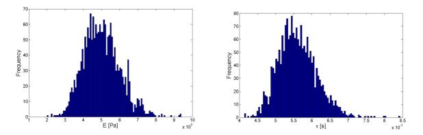
Figure 13: Collision between two discs. Histograms found with Monte Carlo simulations and 2000 realizations. Small deformation case. Left graph: modulus of elasticity; right graph: time of contact.
