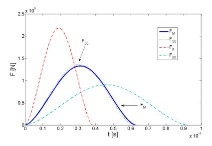
Figure 8: Impact force during contact for the bounds 5%, 50% and 95% and the expected value  $F_M$ .
