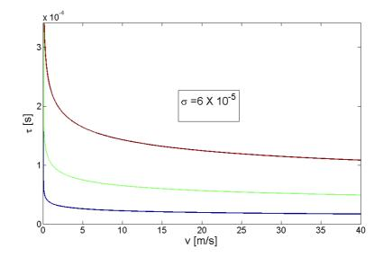
Figure 7: Curves  $\tau$  vs. v and the 5% y 95% bounds for a dispersion  $\sigma_{\alpha} = 6 \ 10^{-5}$ .
