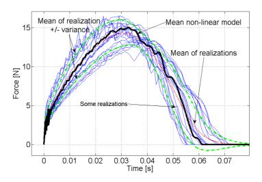
Figure 17: Temporal variation of the contact force. Case 1. Modulus of elasticity  $E(\text{gamma PDF}) \mu_E = 1 \ 10^7 \text{ Pa.}$  $\sigma_E = \mu_E/5$ . Poisson's ratio with uniform PDF. Some randomly chosen realizations (blue full lines), mean of the realizations (dashed red) and the simulation of the mean problem (black full line).
