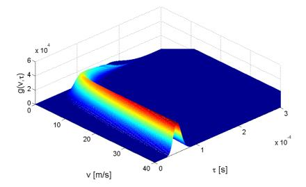
Figure 4: Collision of two steel spheres. Function  $g(v, \tau)$  with  $\sigma_{\alpha} = 2 \ 10^{-5}$ .
