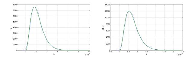
Figure 11: Collision between two spheres. Reconstruction of the PDFs from the numerical simulations using Monte Carlo method. Full lines: distributions found with the analytical approach. Dashed lines: distributions reconstructed from data of Fig. 10.
