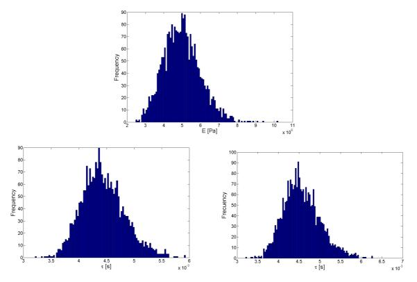
Figure 15: Collision between two discs. Histograms found with Monte Carlo simulations and 2000 realizations. Top graph: modulus of elasticity; lower left graph: time of contact for the small deformations example (v = 10 m/s); right graph: time of contact for the large deformation example (v = 100 m/s).
