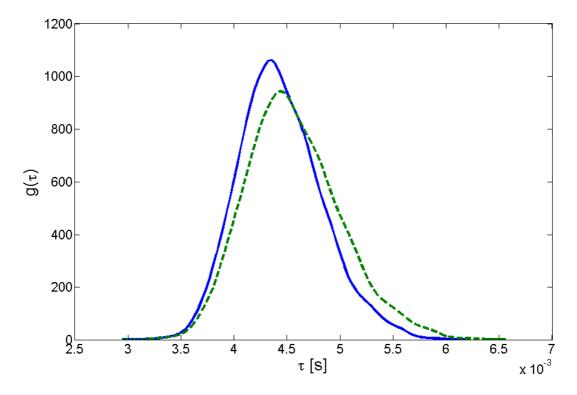
Figure 16: Collision between two discs at v = 100 m/s. Reconstruction of the time of contact PDFs from the numerical simulations using Monte Carlo method reconstructed from data of the lower graphs of Fig. 15. Full line: result from the linear theory; dashed line: result from the finite deformation theory.
