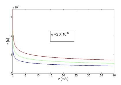
Figure 5: Curves  $\tau$  vs. v and the 5% y 95% bounds for a dispersion  $\sigma_{\alpha} = 2 \ 10^{-5}$ .
