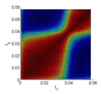
Figure 20: Idem Fig.17. Autocorrelation coefficient. Blue color corresponds to the value -1 (fully anticorrelated). Red color corresponds to the value 1 (fully correlated).
