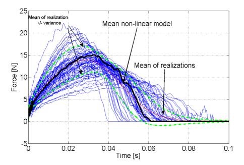
Figure 21: Temporal variation of the interaction force. Case 2. Modulus of elasticity  $E(\text{gamma PDF}) \mu_E = 1e7 \text{ Pa.}$  $\sigma_E = \mu_E/5$ . Poisson's ratio with uniform PDF. Ten random realizations (blue full lines), mean of the realizations (dashed red) and the simulation of the mean problem (black full line).
