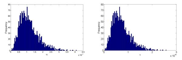
Figure 10: Collision between two spheres. Histograms found with Monte Carlo simulation and 2000 realizations. Left graph: parameter  $\alpha$ ; right graph: time of contact  $\tau$ .
