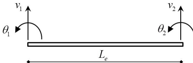
Figure 2: Bernoulli-Euler beam-column finite element with 4 degrees of freedom.
