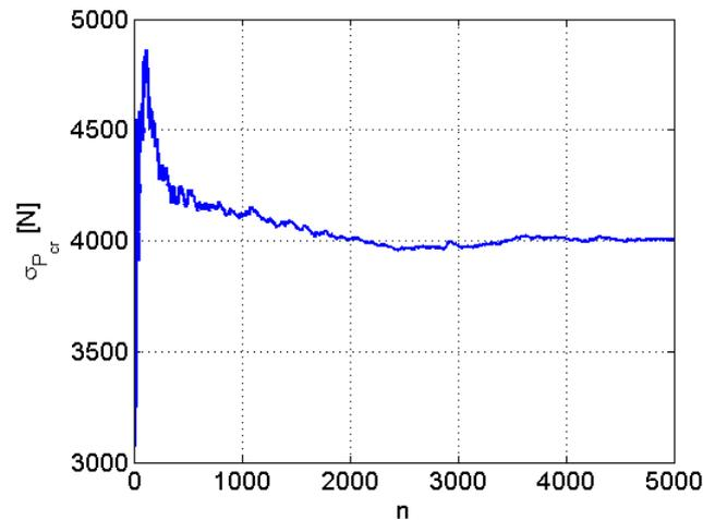
Figure 5: Deviation standard ( $\sigma_{P_{cr}}$ ) convergence for  $\lambda = 110$ .
