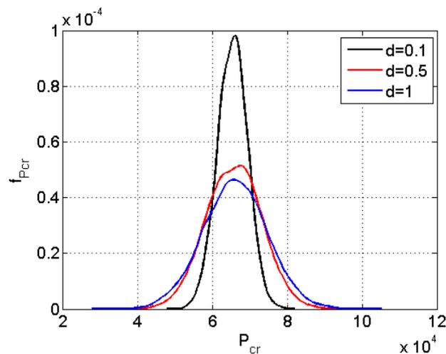
Figure 6: PDF of  $P_{cr}$  for different values of the correlation length  $d$ .
