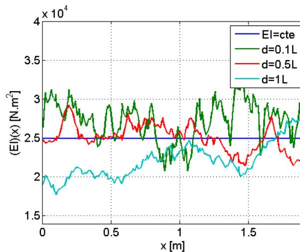
Figure 3: Realizations of the random field  $EI$  for different values of the correlation length  $d$ ,  $\lambda = 110$ .
