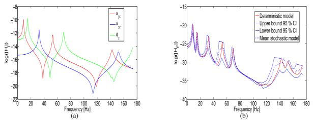
Figure 6: FRFs of the beam with  $\{15, -15, 15, -15\}_S$  stacking sequences ( $\Delta = 5^o$ ). (a) Kinematic variables:  $u_{yc}$ ,  $u_{zc}$  and  $\phi_x$  (b) Displacement of the point where the load is applied.
