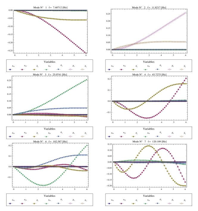
Figure 9: Selected modes shapes of the I-beam with CUS laminate.
