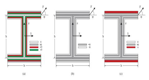
Figure 2: I-beam cross-section profile: (a) quasi-isotropic laminate, (b) angle-ply laminate (c) CUS laminate.
