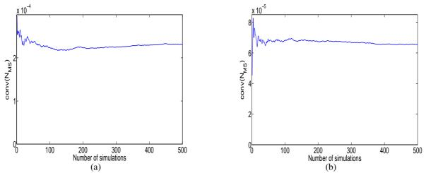
Figure 3: Convergence of the Monte Carlo simulations. (a) For  $\{45, -45, 45, -45\}_S$  stacking sequences, (b) For quasi-isotropic stacking sequences.
