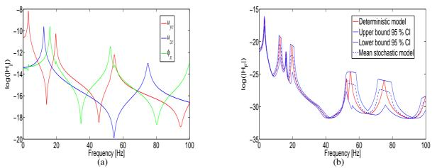
Figure 5: FRFs of the beam with  $\{45, -45, 45, -45\}_S$  stacking sequences ( $\Delta = 2^o$ ). (a) Kinematic variables:  $u_{yc}$ ,  $u_{zc}$  and  $\phi_x$  (b) Displacement of the point where the load is applied.
