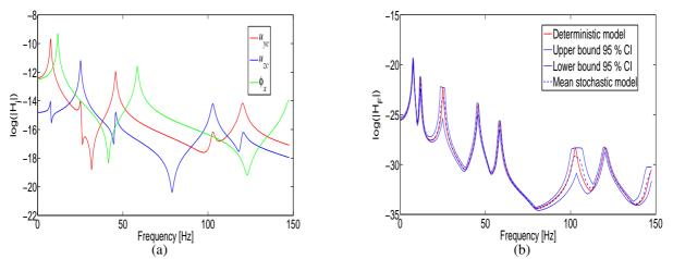
Figure 8: FRFs of the beam with CUS ( $\alpha = 15^{\circ}$ ) stacking sequence ( $\Delta = 5^{\circ}$ ). (a) Kinematic variables:  $u_{yc}$ ,  $u_{zc}$  and  $\phi_x$  (b) Displacement of the point where the load is applied.
