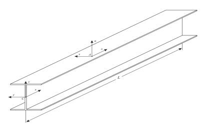
Figure 1: Thin walled beam with reference systems
