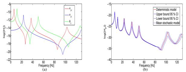
Figure 4: FRFs of the beam with quasi-isotropic stacking sequences ( $\Delta = 2^{\circ}$ ). (a) Kinematic variables:  $u_{yc}$ ,  $u_{zc}$  and  $\phi_x$  (b) Displacement of the point where the load is applied.
