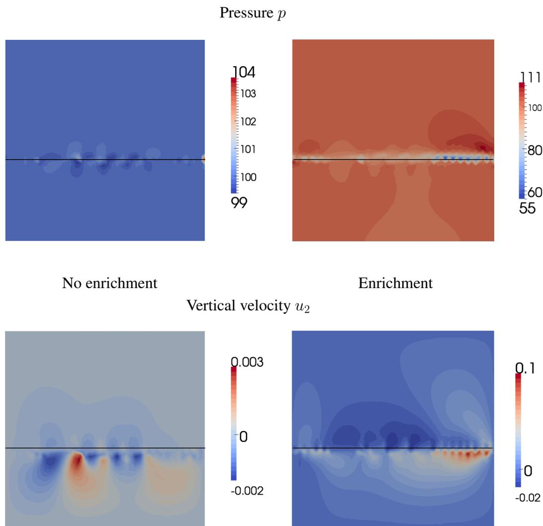
Figure 4: Contours of pressure (top) and vertical velocity (bottom) for the Couette problem without using the enrichment (left) and with the enrichment (right).
