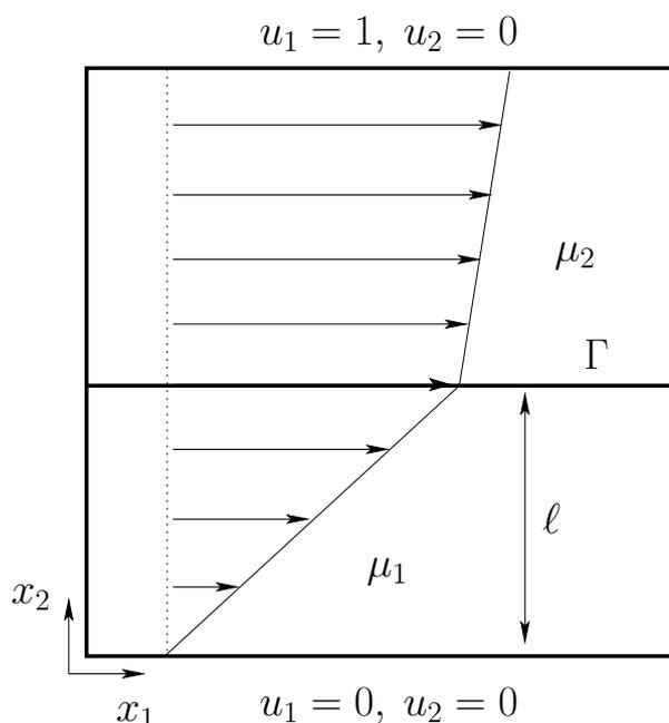
Figure 1: Problem setting for the Couette flow to numerically assess the consistency error of the formulation with the enrichment.
