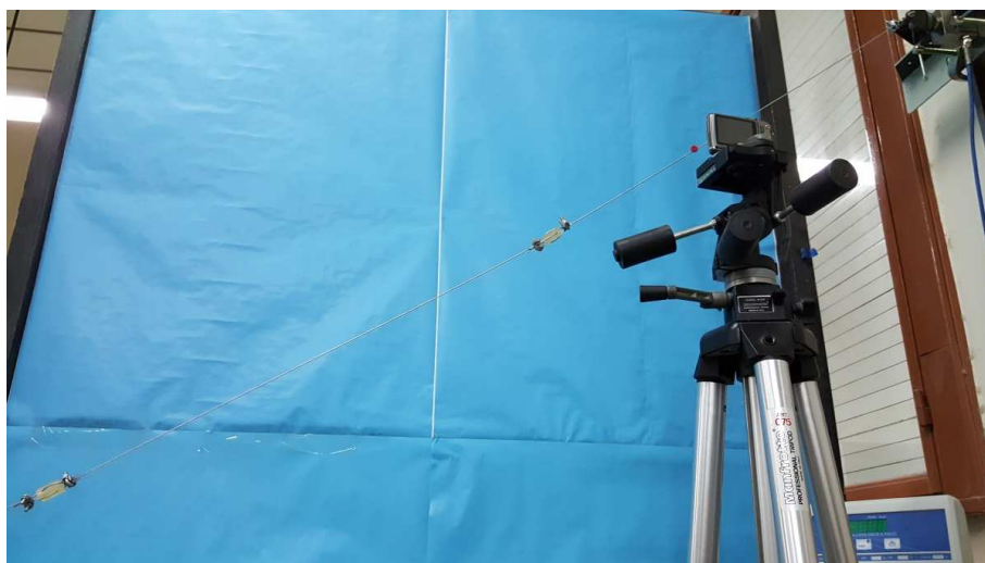
Figure 7: A particular experimental setup of the cable with two insulators.
