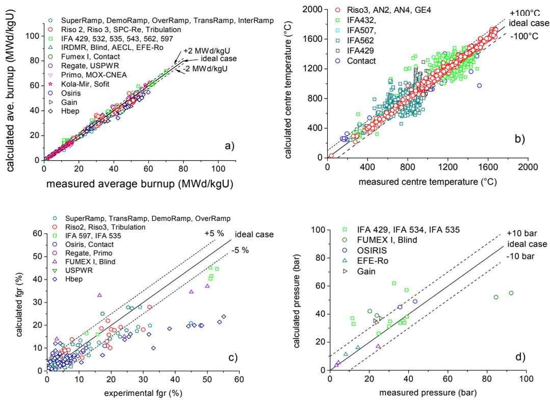
Figure 7: Calculated vs. measured data of a) average burnup, b) centre temperature, c) FGR and d) internal pressure for experiments from IAEA data base
