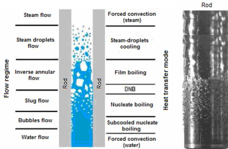
Figure 3: Heat transfer and flow configurations with high heat flux; (In the right) An image of the distribution of convective boiling around a heated rod
