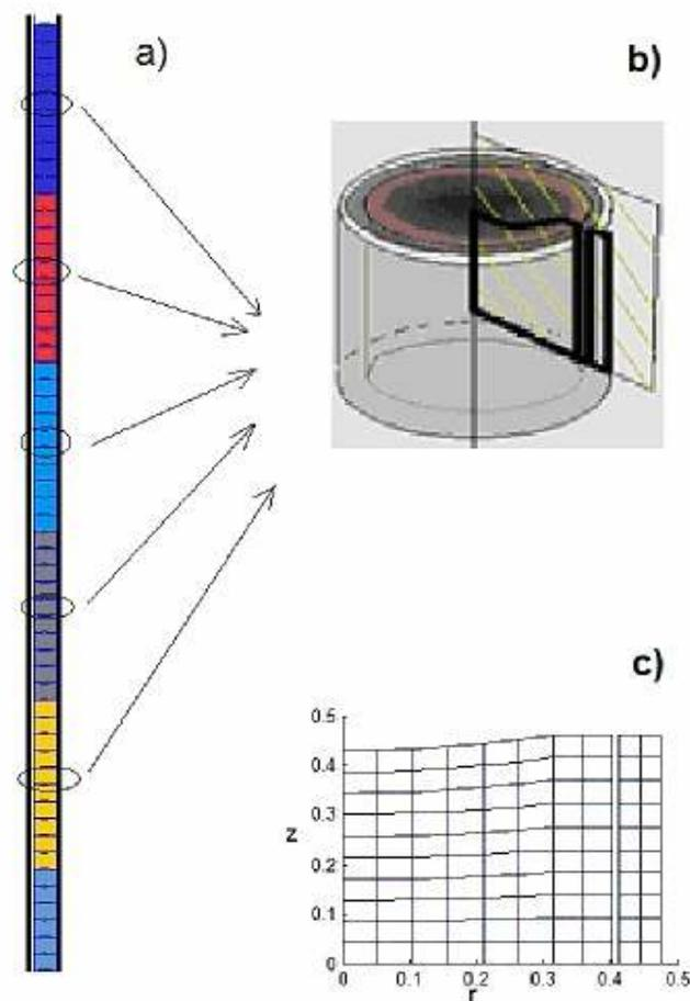
Figure 1: a) Portion of the rod formed by several segments, each one containing a number of pellets. b) One pellet and the corresponding portions of gap and cladding; superimposed is the calculation domain. c) Finite elements discretization of the domain
