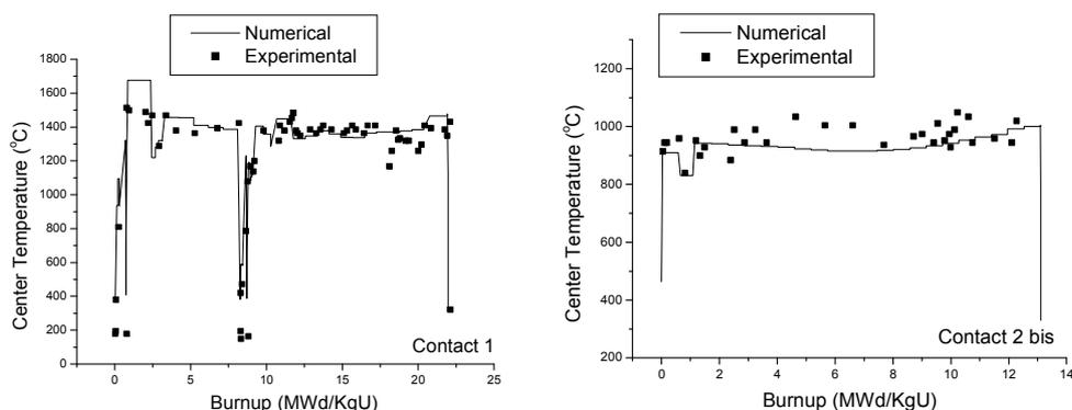
Figure 4: Center temperature for CONTACT 1 and 2bis experiments
