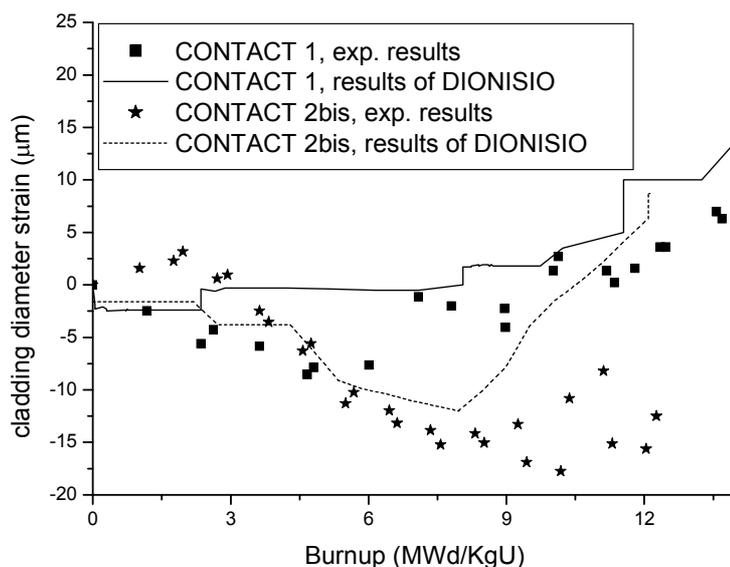
Figure 5: Cladding strain for CONTACT 1 and 2bis
