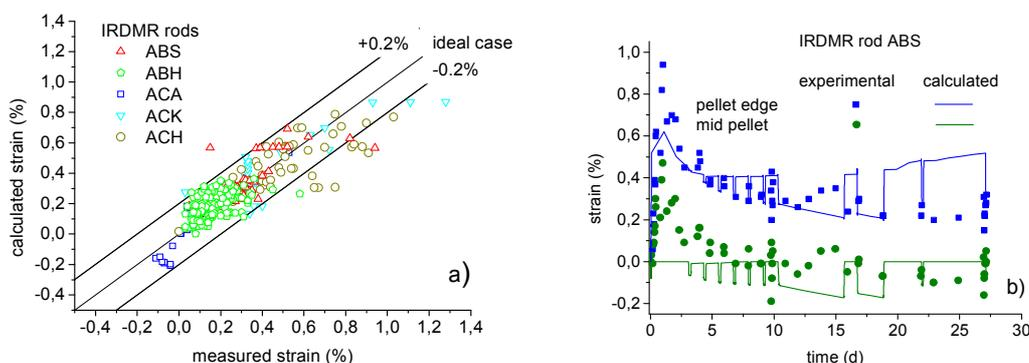
Figure 8: a) Comparison between measurements and the predictions of DIONISIO for several rods of the IRDMR experiment. b) Evolution of the strain at the pellet edge and mid-plane of the ABS rod of the IRDMR experiment
