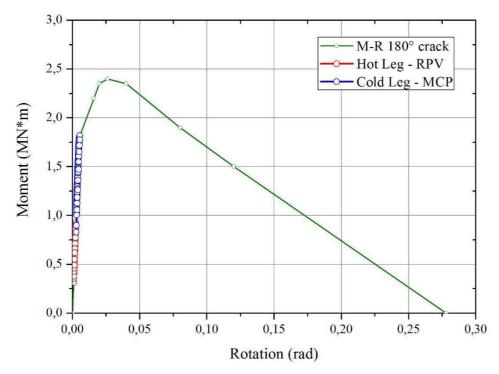
Figure 16: Moment vs Rotation curve for a 180° crack.
