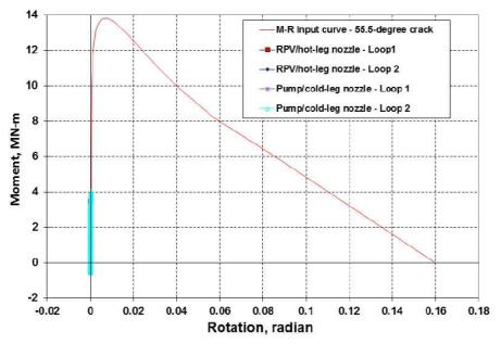
Figure 18: Moment vs Rotation for a 55.5° crack. Engineering Mechanics Corporation of Columbus (2013).
