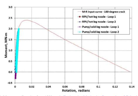
Figure 19: Moment vs Rotation for a 180° crack. Engineering Mechanics Corporation of Columbus (2013).
