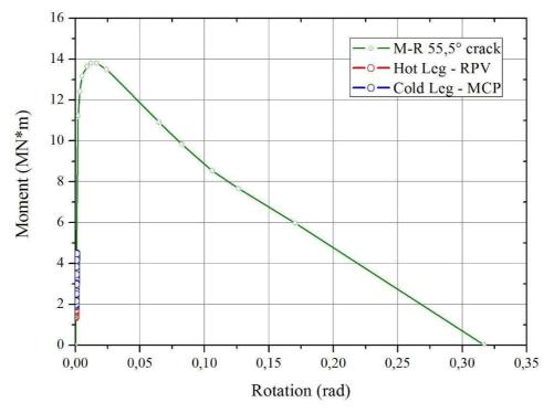
Figure 15: Moment vs Rotations for a 55.5° crack.
