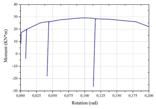
Figure 14: Moment vs Rotation, using a CPE to reproduce IPIRG experiment 1.1-3.
