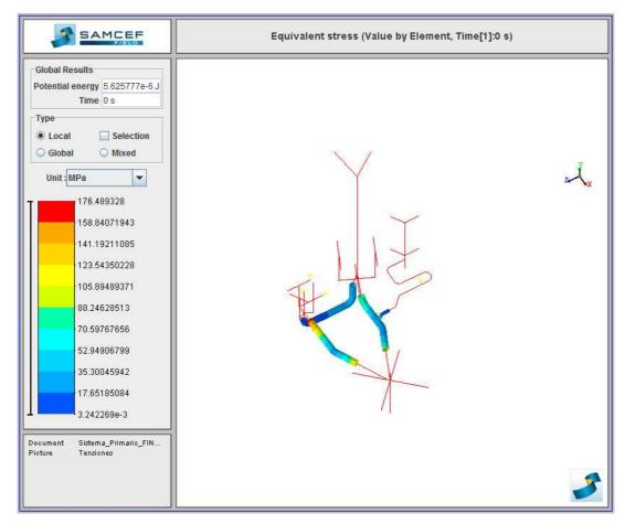
Figure 8: Equivalent stresses in reactor coolant line.
