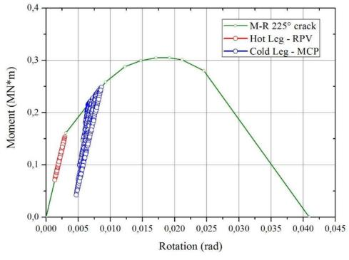
Figure 17: Moment vs Rotation for a 225° crack.
