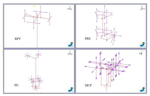
Figure 7: Application of the displacement time histories.
