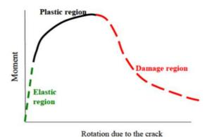
Figure 10: Moment vs Rotation due to the crack.
