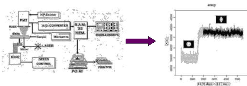
Figure 1. Flowchart of Erythrocyte Rheometer and a typical time series from the creep process of
