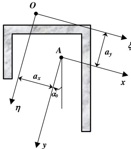
Figure 6: Principal axes of channel unnsymmetrical beams.
