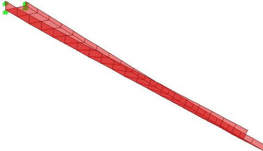
Figure 7: Mode 2. Beam 1. Clamped-Free. Software SAP2000.
