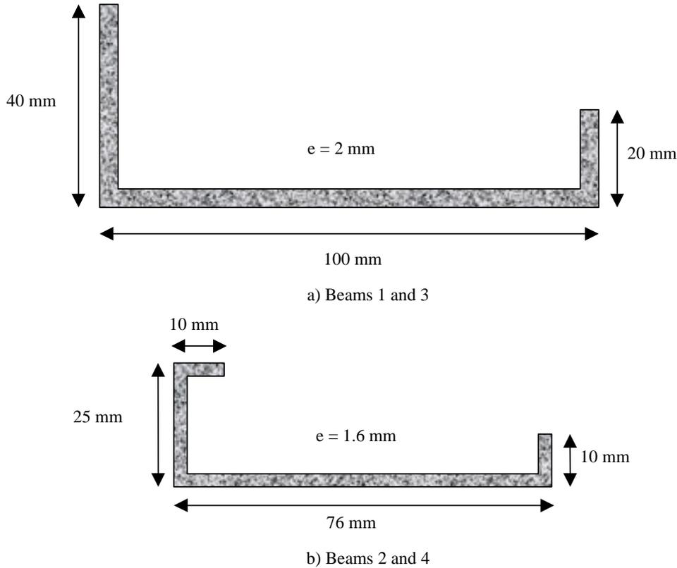
Figure 2. Cross-section of the beams tested
