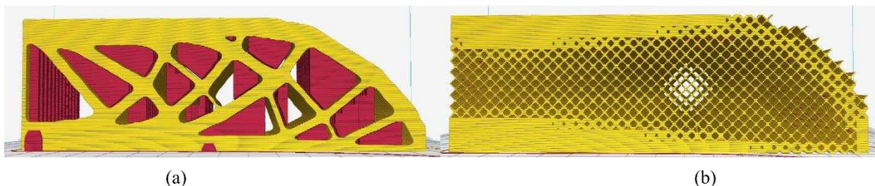
Figure 6 Solid and lattice printing simulation giving by Ultimaker Cura (Braum, 2018).
