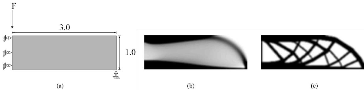
Figure 4: MBB problem: (a) geometry and boundary conditions, (b) TO with  $p = 1$  (c) TO with  $p = 1 - 3$
