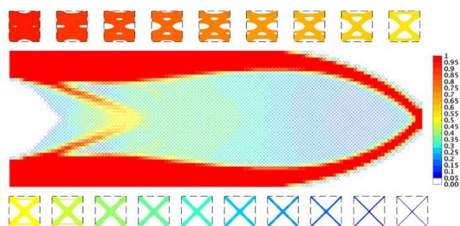
Figure 3: Optimization result for a cantilever beam (Li et al., 2018).
