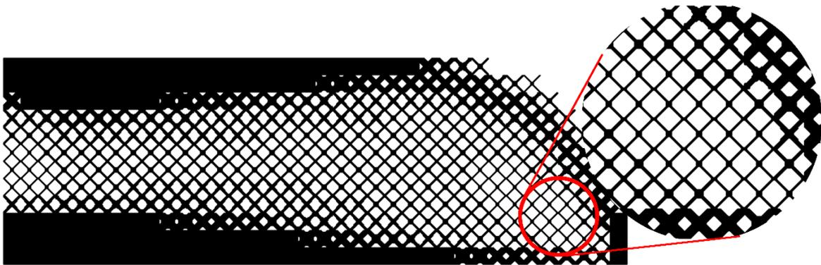
Figure 5: Lattice solution using the variable-density method.
