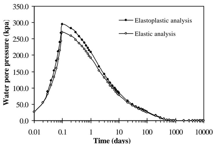
Figure 5: Evolution of pore pressure
