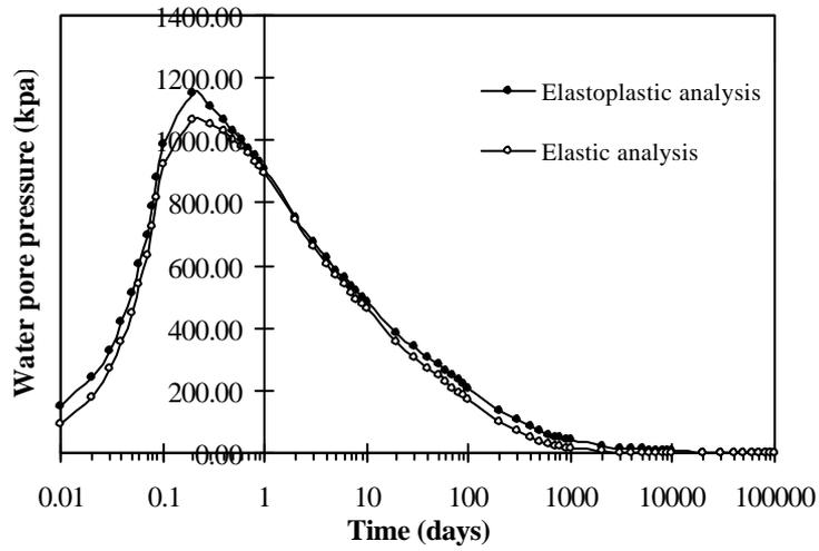
Figure 7: Disipation of water pore pressure
