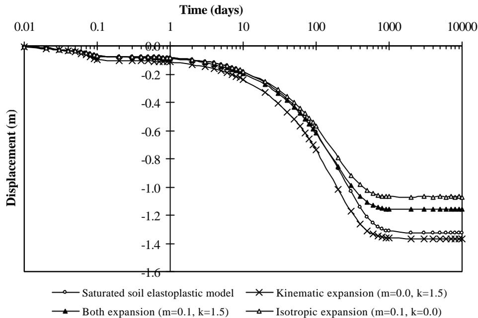
Figure 6: Displacement vs. time for different plastics parameters of the yield criterion
