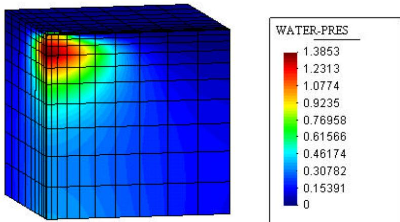
Figure 9: State of the water pore pressures to the second day and finite element mesh
