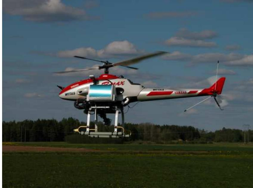
Figure 4: Drone: Helicopter RMAX Yamaha.
