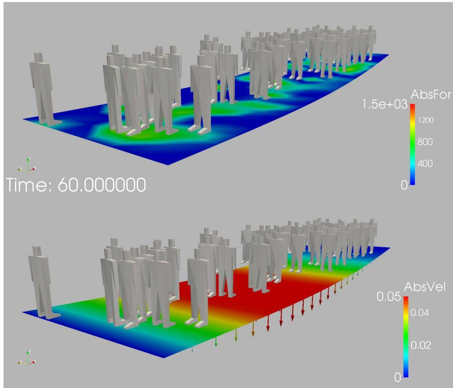
Figure 2b Force and Velocities of the Structure at T=60 sec
