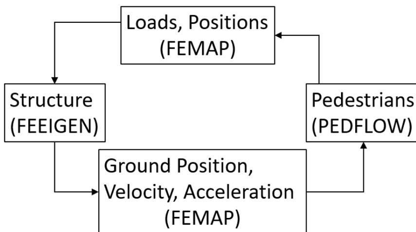
Figure 1 Loose Coupling of CSD and CCD Codes
