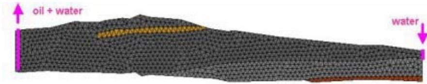
Figure 3. Finite element mesh used in the analysis (1907 elements and 1046 nodes).
