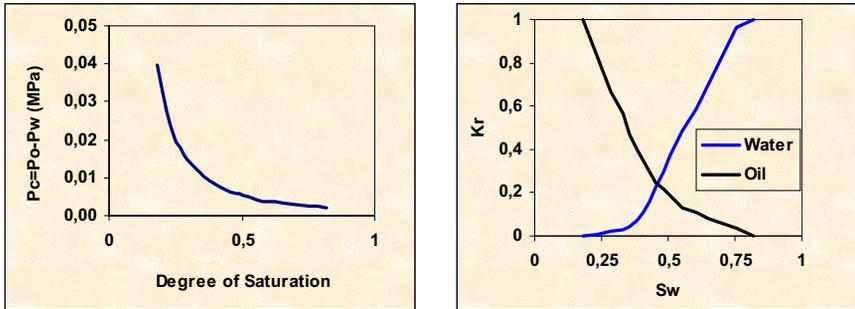
Figure 2. Material parameters for hydraulic problem: (a) retention curve and (b) relative permeability ( $k_r$ ) curve.
