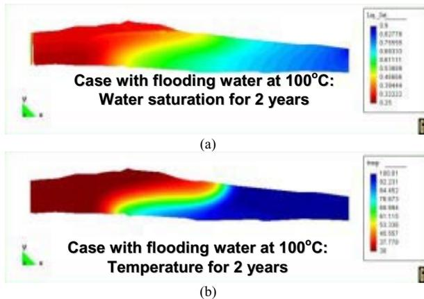
Figure 10. (a) Water saturation and (b) temperature distribution for 2 years analysis.
