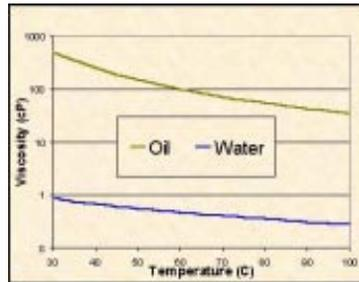
Figure 7. Oil and water viscosity as function of temperature.
