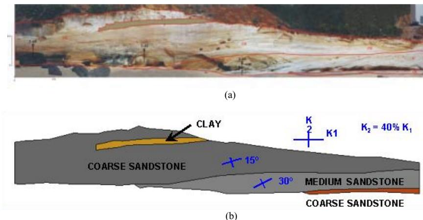
Figure 1. Barreiras de Boqueirão outcrop: (a) Photomontage; (b) numerical model geometry for multiphase flow in the Analogous.
