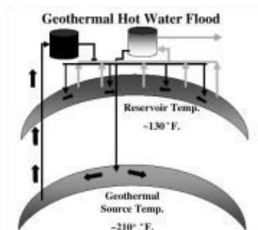
Figure 6. Schematic drawing of hot water flooding, from a geothermal source in a heavy oil reservoir<sup>6</sup>.
