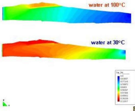
Figure 8. Water saturation distribution after 5 years water flooding at different temperatures (100 e 30°C).
