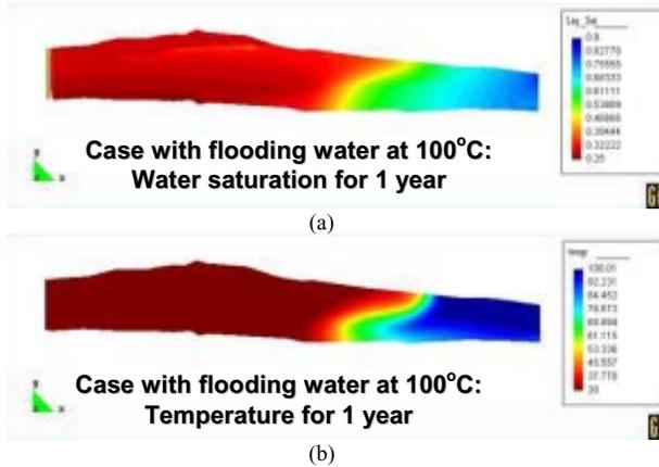
Figure 9. (a) Water saturation and (b) temperature distribution for 1 year analysis.
