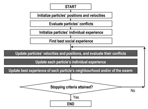
Figure 1: General flowchart for the whole PSO algorithm.
