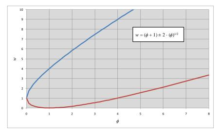
Figure 3: Regions in the ' $\phi$ –w' plane corresponding to each of the three cases of  $\gamma$ . The points on the parabola correspond to  $\gamma^2 = 0$ ; the region inside the parabola corresponds to the complex conjugates roots; while the remainder of the plane corresponds to two different and real-valued roots.
