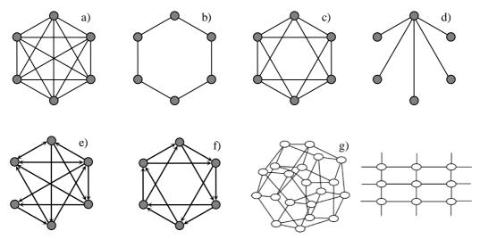
Figure 2: a) *global* topology; b) *ring* topology with two neighbours; c) *ring* topology with four neighbours; d) *wheel* topology; e) *random* topology; f) *forward* topology with two neighbours (from Innocente (2010)); g) *von Neumann* topology (from Kennedy and Mendes (2006)). No arrow means that the link is bidirectional.
