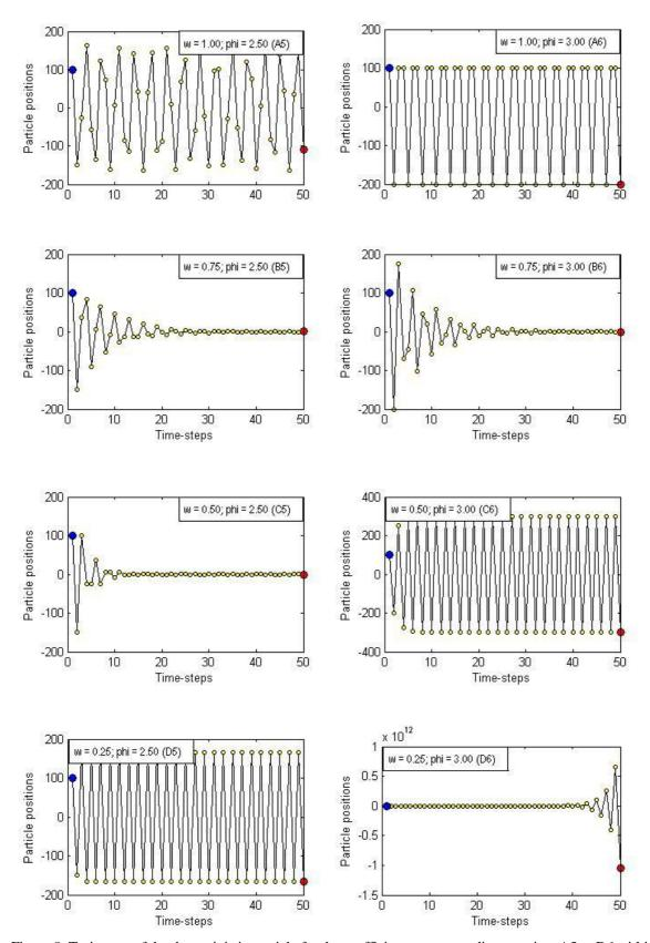
Figure 8: Trajectory of the deterministic particle for the coefficients corresponding to points A5 to D6 within Sub-region III in Figure 5.
