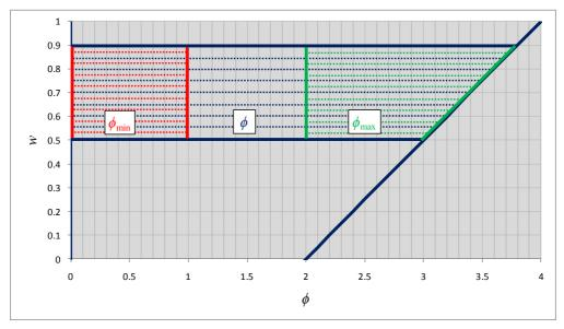
Figure 9: Suggested region in the ' $\phi$ –w' plane from where  $\phi$  is to be randomly sampled (blue dotted lines). The regions of suggested upper ( $\phi$ <sub>max</sub>) and lower ( $\phi$ <sub>min</sub>) limits of  $\phi$  are shown in green and red dotted lines, respectively.
