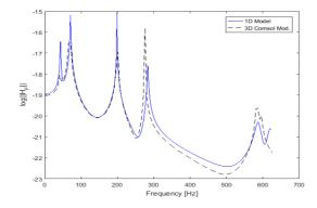
Figure 2: FRF of the present 1D curved beam and COMSOL 3D.
