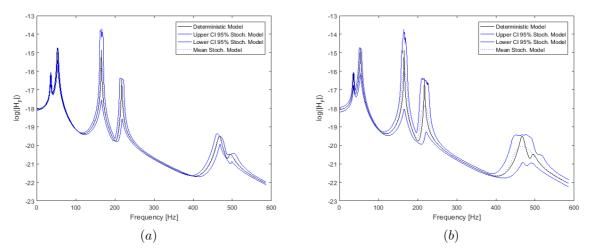
Figure 4: Confidence intervals for CoV = 0.1. (a) For the random variable  $\Gamma_c$ , (b) All random variables.
