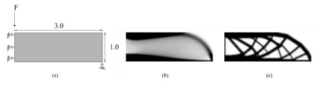
Figure 4: MBB problem: (a) geometry and boundary conditions, (b) TO with p = 1 (c) TO with p = 1 - 3
