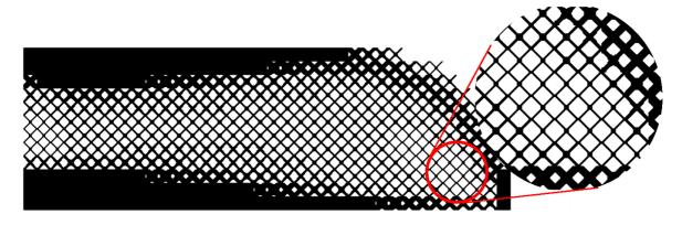
Figure 5: Lattice solution using the variable-density method.
