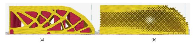
Figure 6 Solid and lattice printing simulation giving by Ultimaker Cura (Braam, 2018).
