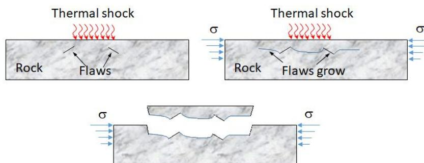
Figure 1: Principle of thermal spallation.
