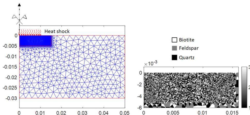
Figure 2: The CST mesh (7961 elements, the unit of the dimensions is m), boundary conditions, and the numerical rock mineral structure.
