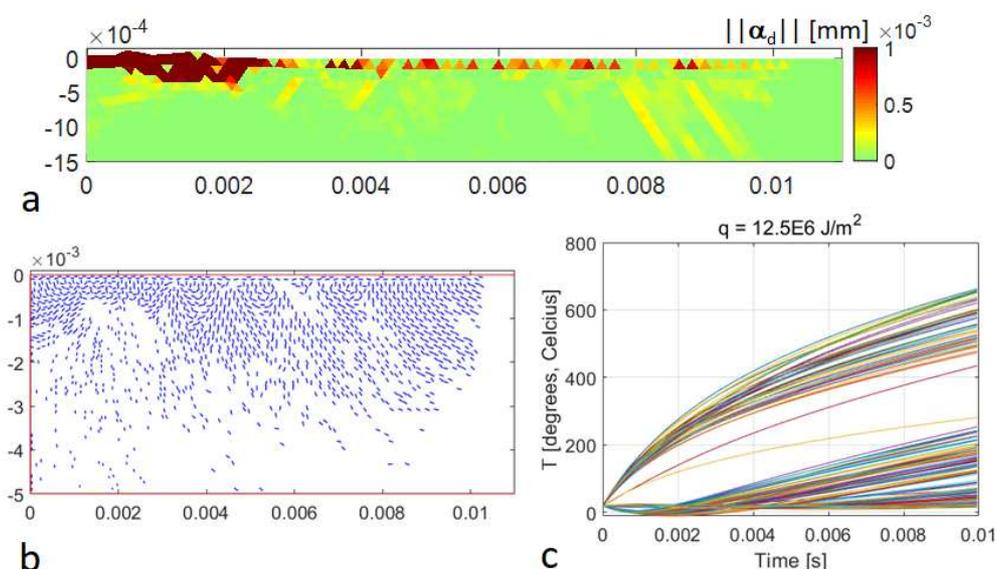
Figure 4: Simulation results for the thermal spallation of rock under a constant heat flux  $q_n = 12.5E6 \text{ J/m}^2$ : the magnitude of crack opening vectors (a), the crack orientations (b) at the end of simulation, and the temperature evolution at all nodes of the rock sample (c).
