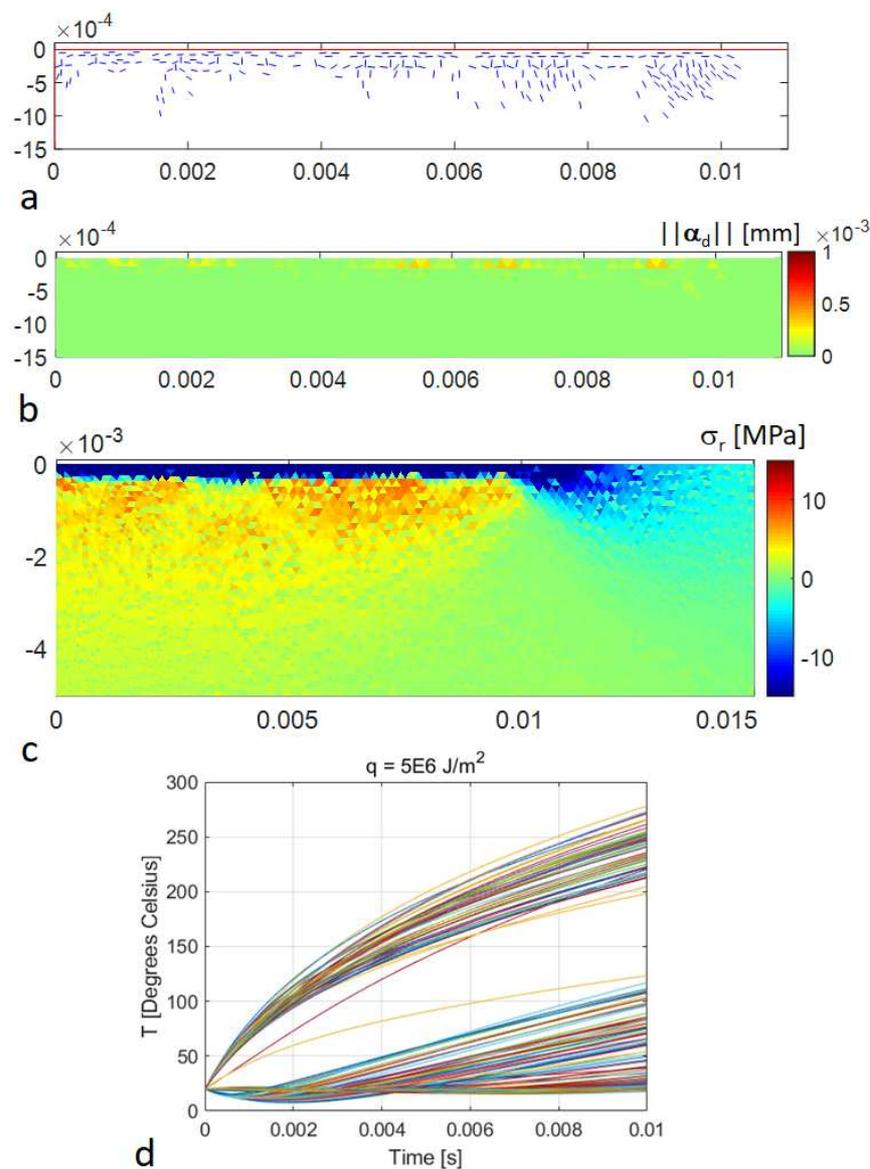
Figure 3: Simulation results for the thermal spallation of rock under constant heat flux  $q_n = 5E6 \text{ J/m}^2$ : the crack orientations (a), the magnitude of crack opening vectors (b), the radial stress distribution (c) at the end of simulation, and the temperature evolution at all nodes of the rock sample (d).
